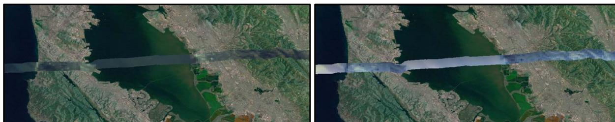
Figure 8. Segment of a flight track over San Francisco Bay. The area shown is 60km x 30km. SPEX airborne data from the nadir viewport is the narrow strip (2.5km wide swath), plotted over a reference image from World Imagery from ArcGIS, ESRI. Left image displays RGB radiance, right panel shows RGB polarization (DoLP).
