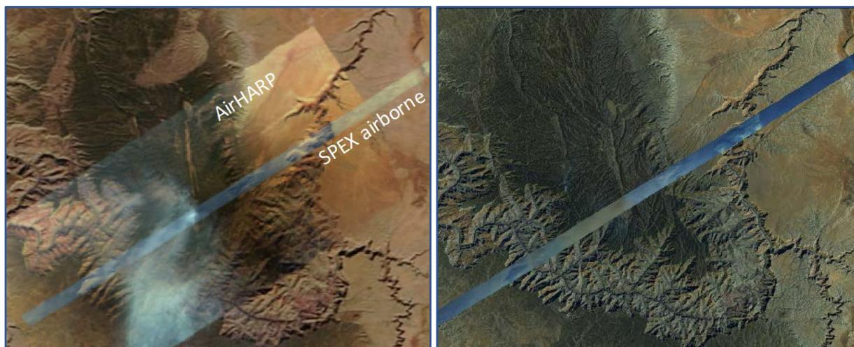
Figure 9. Flight track over Grand Canyon, capturing a smoke plume from a forest fire. The area shown is 80km x 80km. Left image displays RGB radiance, right panel shows RGB polarization (DoLP). The left image includes a pushbroom-color image from AirHARP, with the SPEX airborne strip overlaid. The background image from MODIS of the same day.
