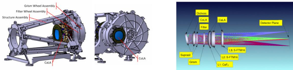
Figure 1-1 Near Infrared Spectro-Photometer (NI-SP) opto-mechanical design (left) and optical layout (right)
