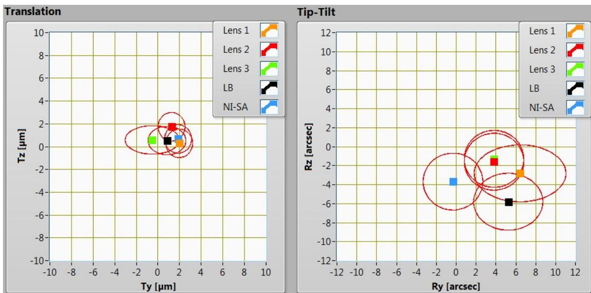
Figure 5-3: CaLA EQM translation and displacement (Tip-Tilt) of Lens 1-3, LB and NI-SA in z- and y-direction with correction values for the setup and error circles.
