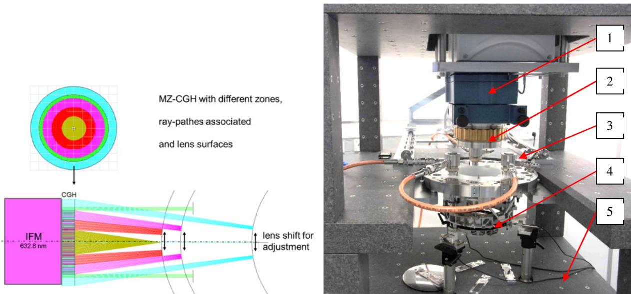
Figure 3-1 Alignment concept with Multi-Zonal-CGH (left); right: Interferometric alignment tower: 1: Zygo Interferometer, 2: multi-zone CGH, 3: Hydraulic bolt tensioner for tightening all three fixation bolts of a lens assembly simultaneously in the aligned position, 4: CaLA Structure with L3 and L2, 5: highly stable granite alignment tower
