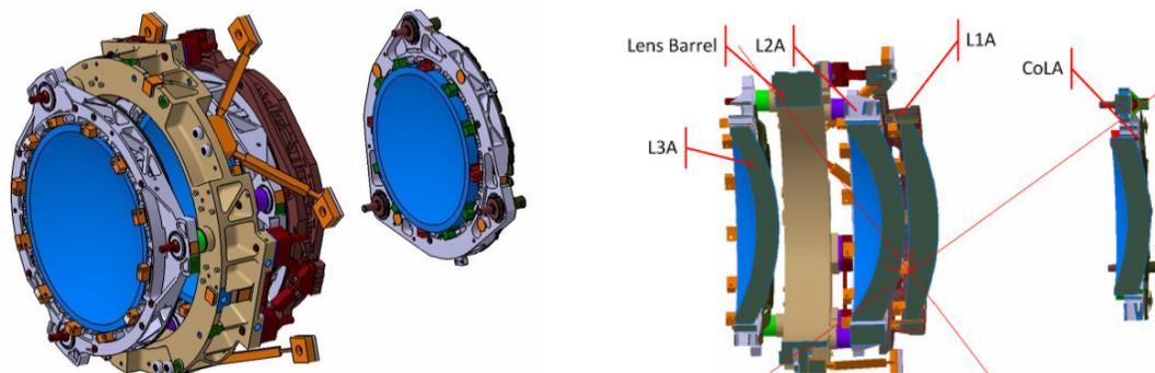
Figure 2-1 3D CAD view of the Near Infrared Spectro-Photometer Optical Assembly (NI-OA) consisting of the CaLA triplet and CoLA (left), cross-section with nomenclature of lens-assemblies (right)
