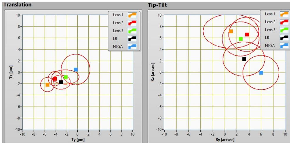
Figure 5-4 CaLA FM Translation and displacement (Tip-Tilt) of Lens 1-3, LB and NI-SA in z- and y-direction with correction values and error circles
