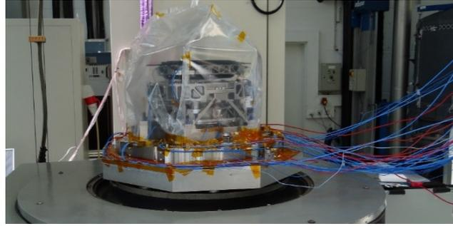
Figure 5-5 CaLA EQM mounted on the shaker at MPE (incl. protection cover for cleanliness)
