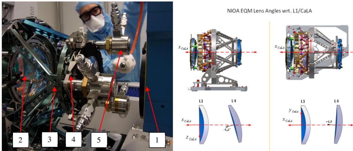
Figure 5-6 left: Assembly and alignment of CoLA lens relative to the CaLA Lens assembly: 1: Interferometer / alignment CGH; 2: L1 of CaLA; 3: Interface dummy between CaLA and CoLA; 4: CoLA Lens assembly; 5: Hydraulic bolt tensioner; right: achieved positional accuracy (tip/tilt) of CoLA relative to the L1 reference surface on CaLA, measured with a CMM.
