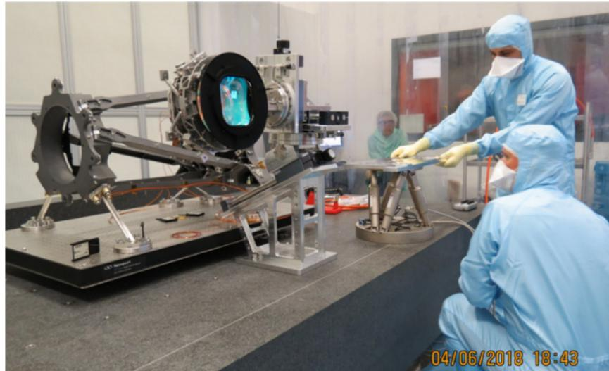
Figure 6-1 CaLA EQM integration to the NISP SIC structure at LAM
