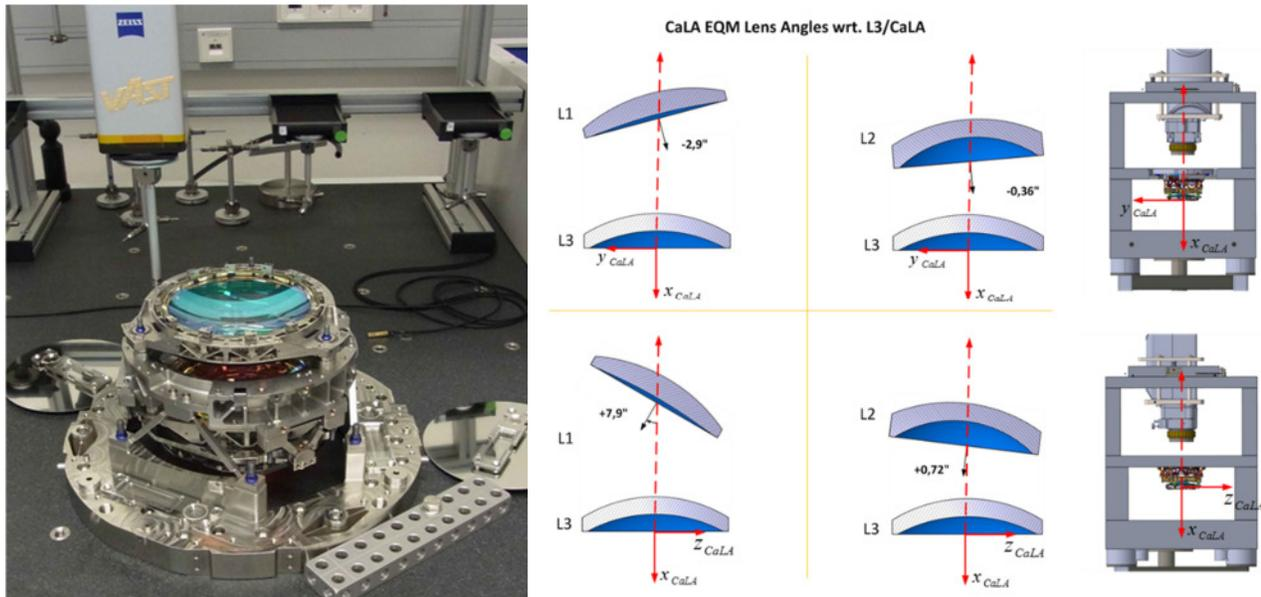
Figure 5-1 left: Coordinate Measurement Machine in ISO 4 environment to characterize the opto-mechanical alignment of CaLA before and after the environmental tests; Right: EQM measurement results, evaluated for tip/tilt angles between the individual lenses
