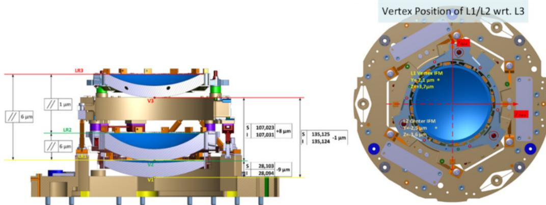
Figure 5-2 left: cross-section of CaLA showing the vertex positions of all three lenses and the relative tilt (parallelism) right: top view to view of CaLA, showing lateral displacement of the L1 and L2 Vertices relative to the L3 Vertex
