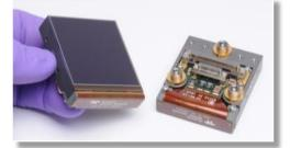
Figure 9: The H4RG-10, 4K×4K pixels, 10 µm pixel pitch
