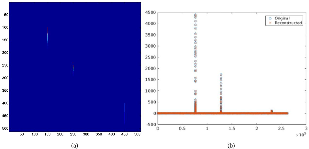
Figure 2: UV-VIS hyperspectral imager: (a) Original synthetic image, and (b) Reconstruction vs. original with CR =10.
