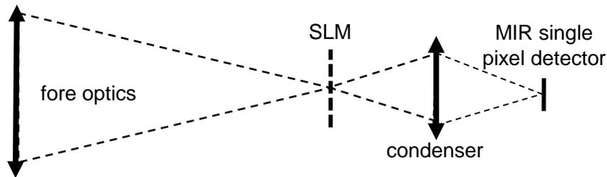
Figure 3. Schematic layout of the camera operating in the MIR-TIR for sky observations and real time detection of NEO.
