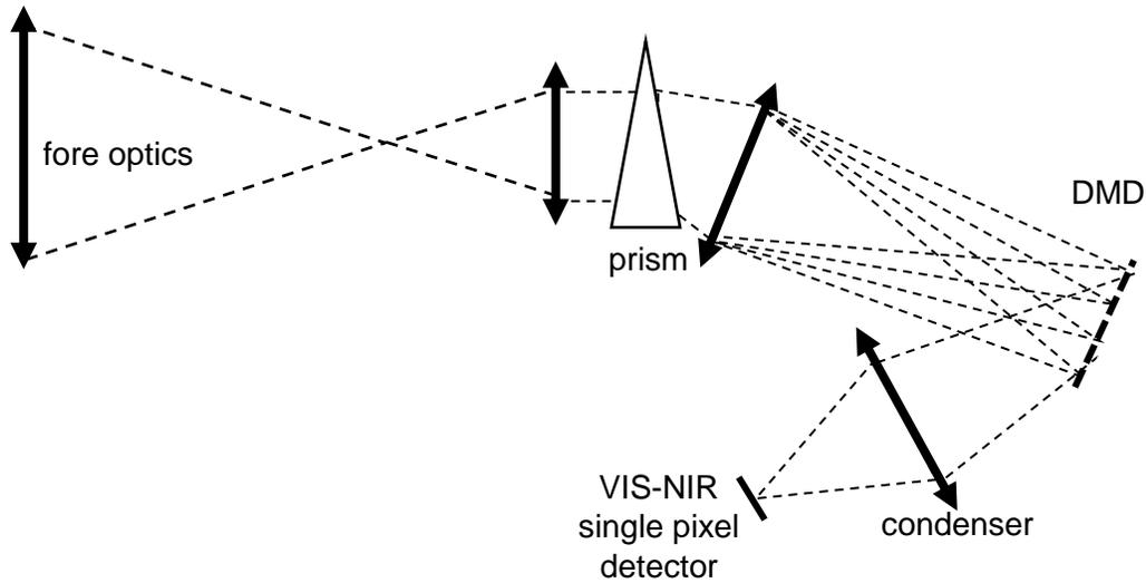
Figure 1. Schematic layout of the UV-VIS hyperspectral imager.
