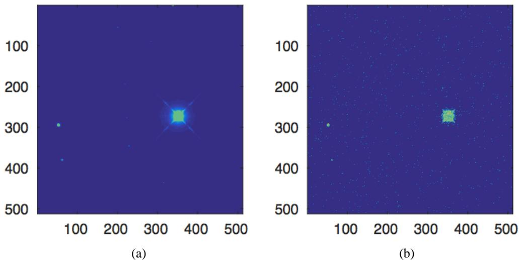
Figure 4. MIR camera (a) Simulated image at the SLM: (a) image with a very large star and few small objects, and (b) Reconstruction from 10% samples using BCCB sensing matrix and OMP.
