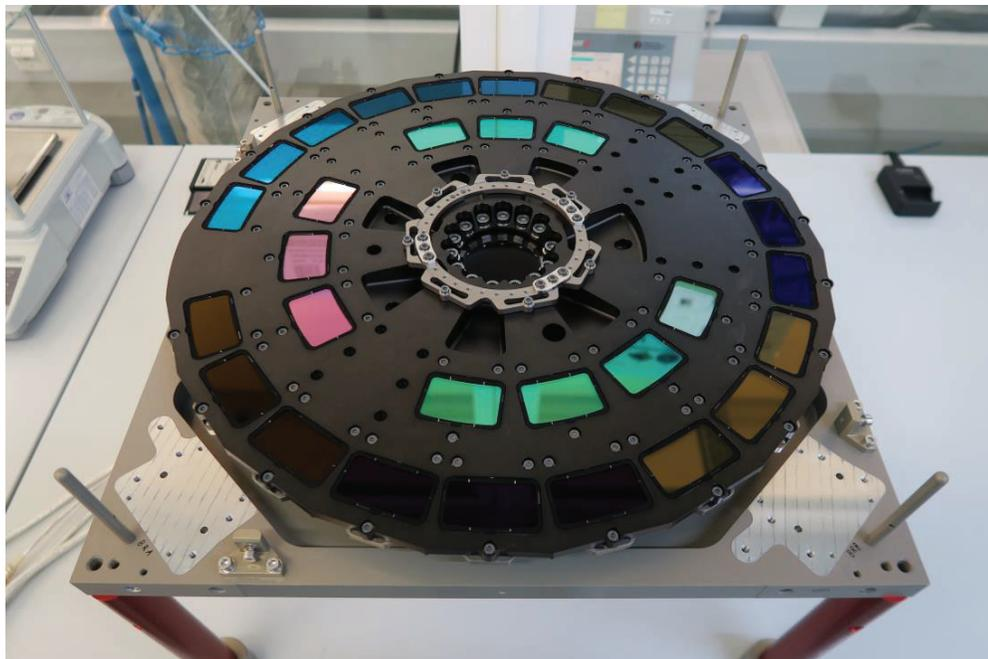
Figure 2. Filter Wheel Assembly (FWA) (Courtesy of RUAG [3]).
