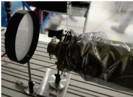
Figure 3 Optical layout of Metis in the laboratory calibration test set-up.
