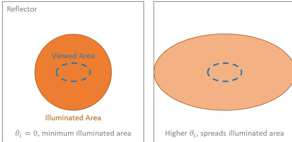
Figure 2. Illustration of a fixed  $\theta_v$  with varying  $\theta_i$ . The same amount of flux lies in the illuminated areas, but it is more dispersed across the spread area for a larger illumination angle  $\theta_i$ .
