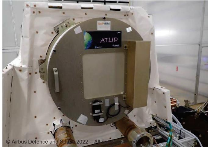
Figure 17: Photo of the receive chain (RxA) IPC OGSE cover mounted on ATLID telescope baffle.
