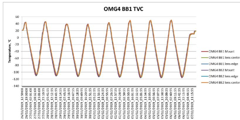
Figure 12. OMG-4 BB1 and BB2 TVC temperature profile.
