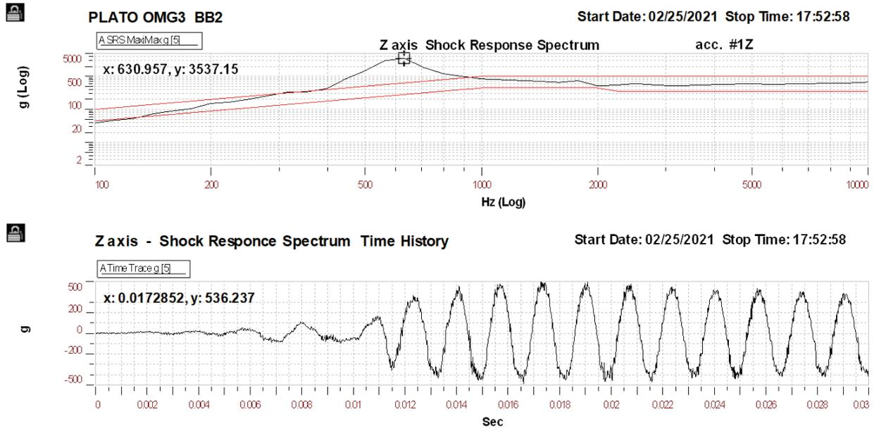
Figure 21. OMG-3 BB2 Shock Z axis 500g – Lens response.
