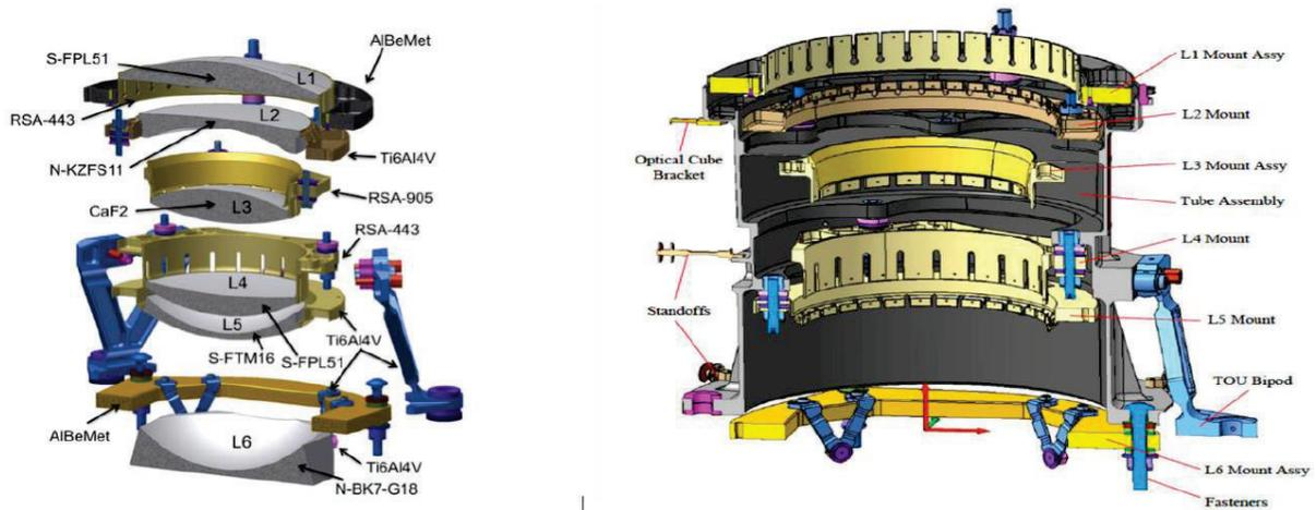
Figure 3. Left: an exploded view of a PLATO's TOU with a focus on the materials used for the glasses, their mounts, and for the interface components. Right: Details of the mechanical structure with subcomponents highlighted.
