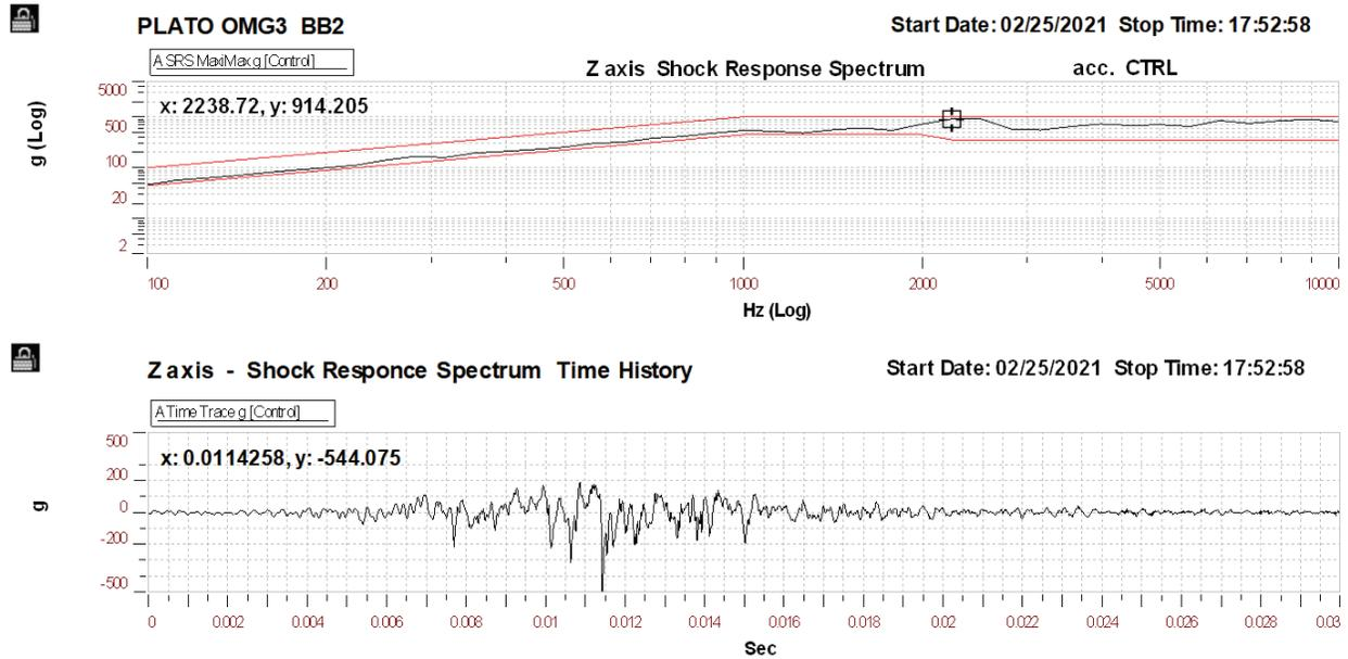
Figure 20. OMG-3 BB2 Shock Z axis 500g - Input.
