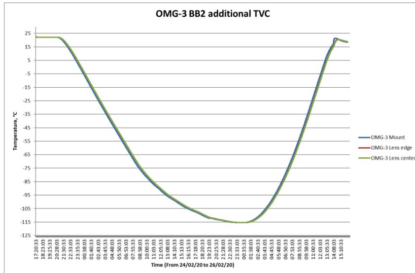
Figure 11. OMG-3 BB2 additional TVC temperature profile.
