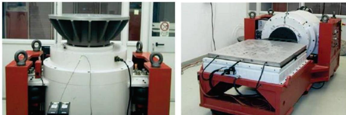
Figure 13. Shaker used for vibration test on BBs.
