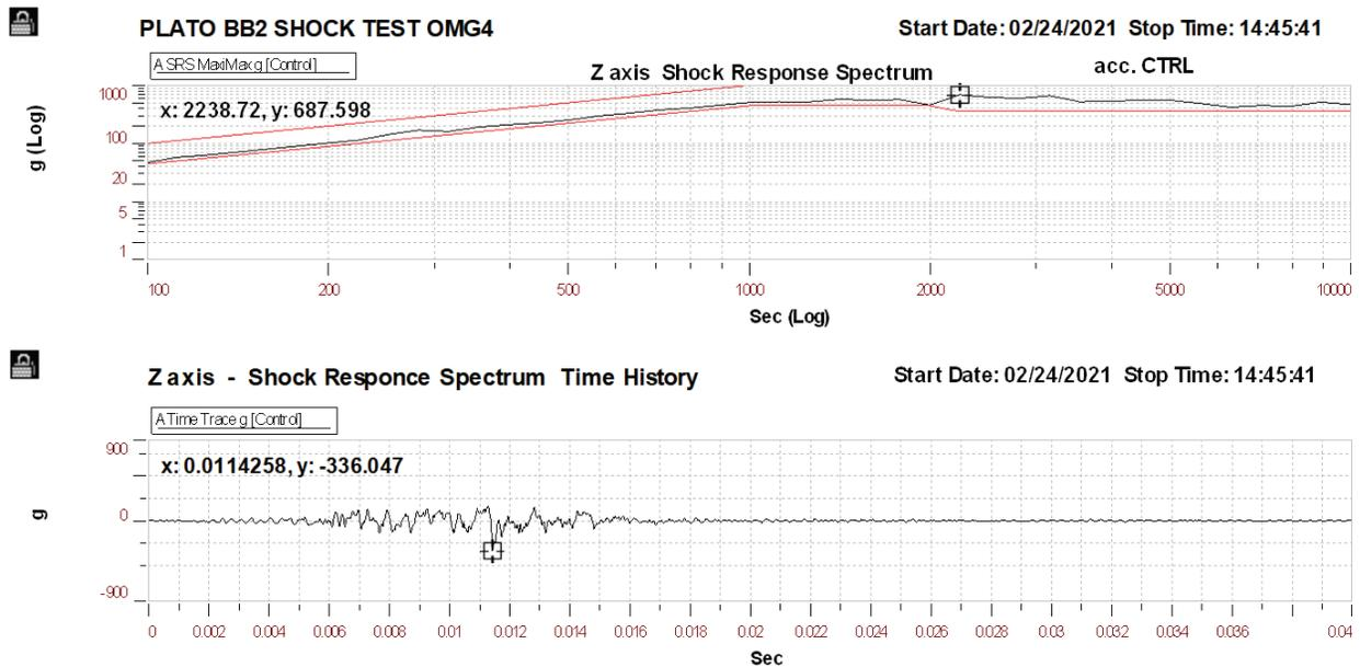
Figure 22. OMG-4 BB2 Shock Z axis 500g - Input.
