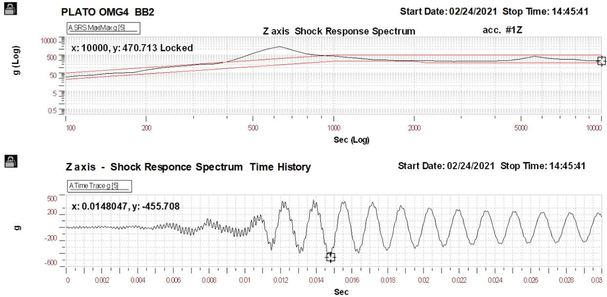
Figure 23. OMG-4 BB2 Shock Z axis 500g – Lens response.
