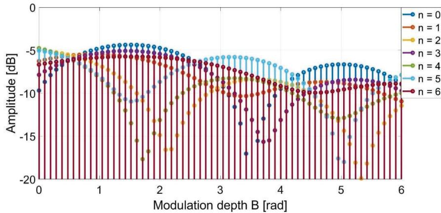
**Fig. 3.** Amplitude of the first six harmonics as a function of the modulation depth of the second sinusoidal signal. The value of 'n' indicates the considered sideband.
