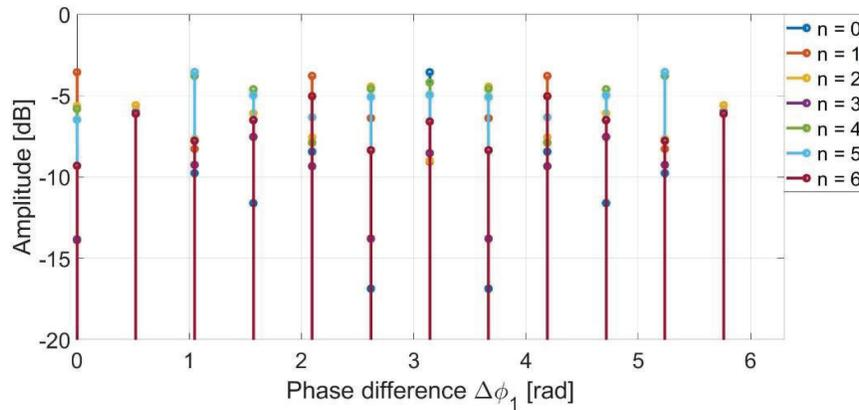
Fig. 2. Amplitude of the first six harmonics as a function of the phase difference between the first signal and the signal chosen as phase reference. The value of 'n' indicates the considered sideband.
