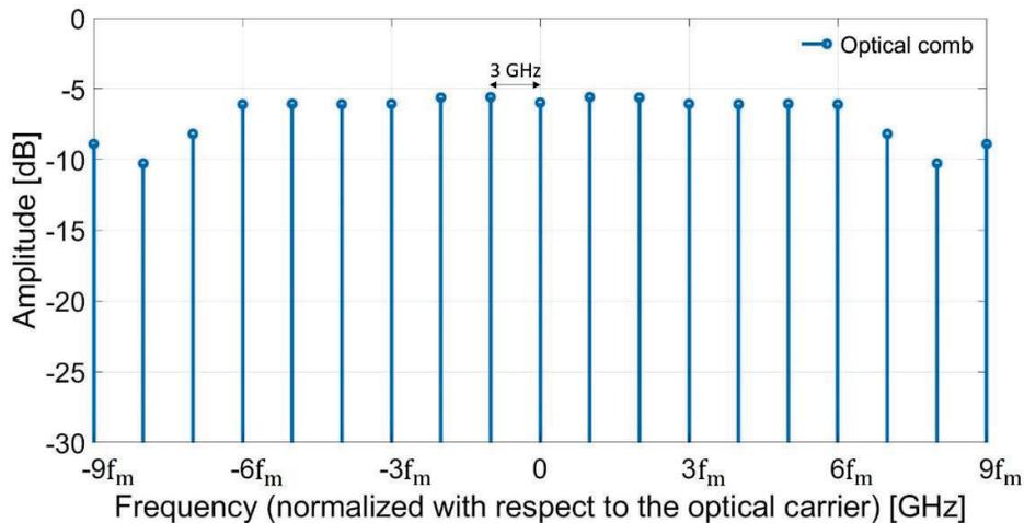
**Fig. 4.** Output spectrum showing the generated ultra-flat 13 lines and 3 GHz spacing OFC. The amplitude difference between the strongest and the weakest line of the comb is 0.5 dB.
