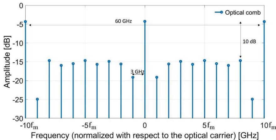
**Fig. 6.** Heterodyne output signal generated by driving the modulator with three RF signals. The extinction ratio between the desired tones and the undesired ones is always higher than 10 dB.
