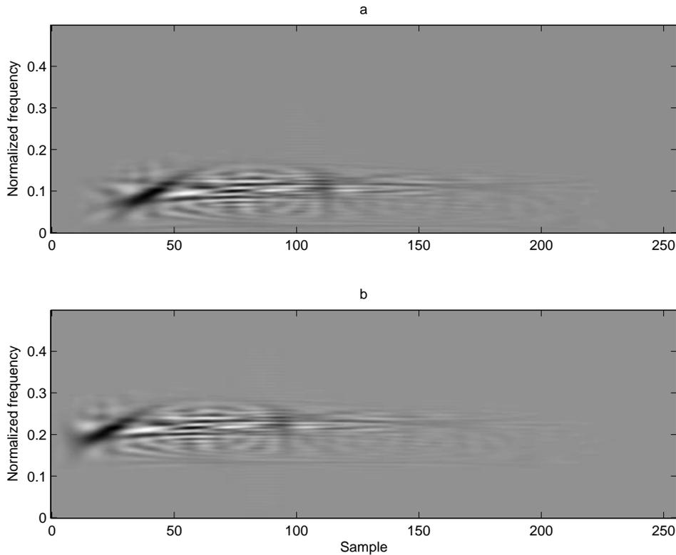
**Figure 3.** TFDs of a. original, b. frequency shifted click
