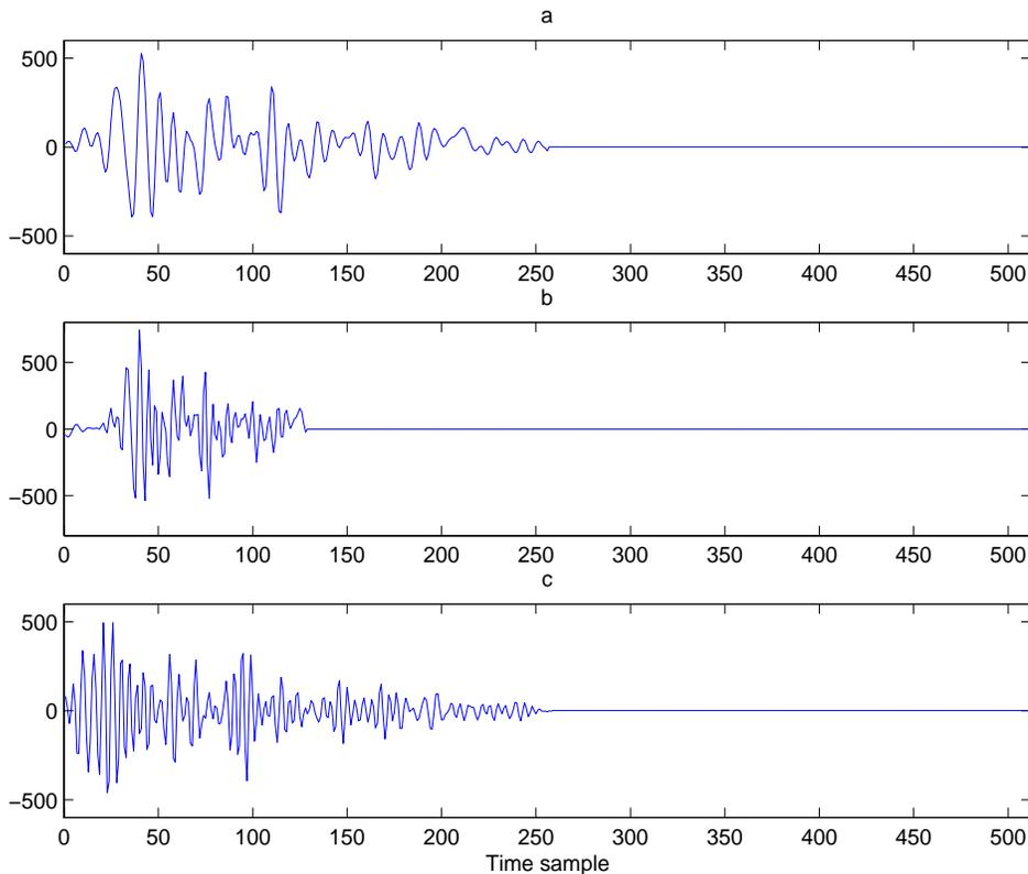
**Figure 1.** Example of a. original, b. scaled and c. frequency shifted click
