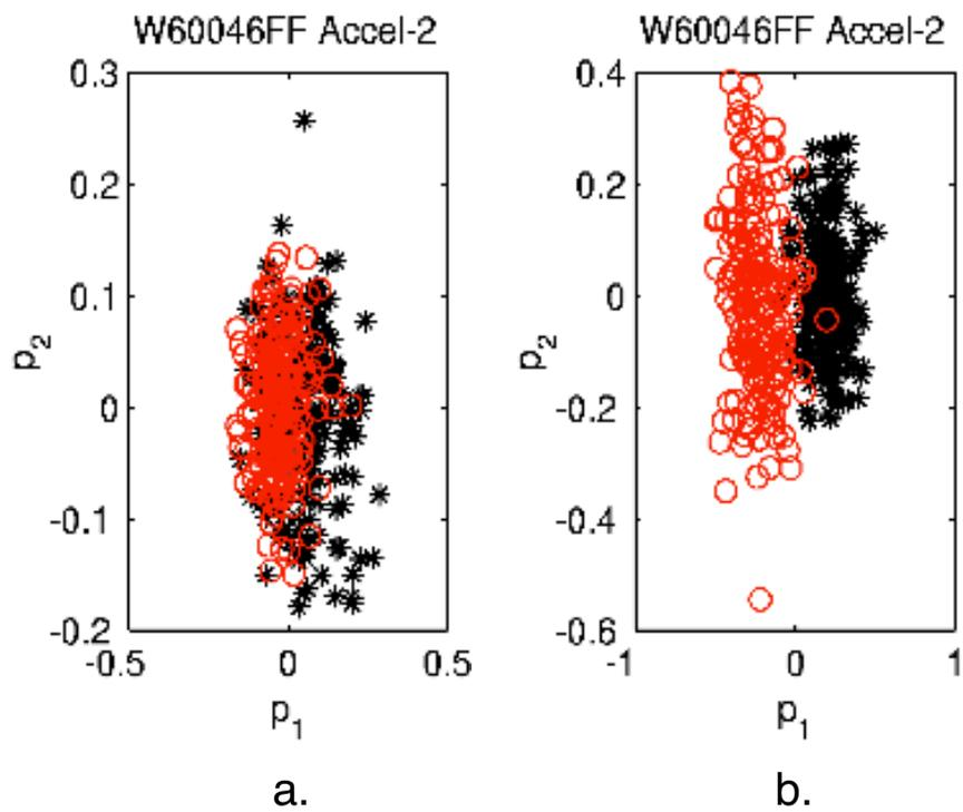
**Figure 7.** Scatter plots for a. scale transformed spectra, b. spectra with circles showing faults
