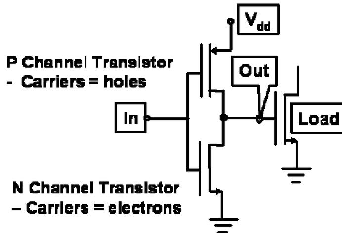
Figure 1. Simple Inverter Circuit showing a transistor load on the out line.
