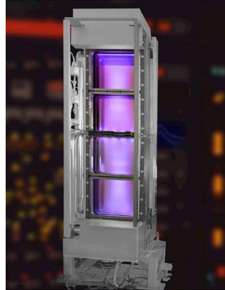
Fig 2. KDP doubler crystal grown using the rapid growth technique (left image). Final assembly of the PEPC utilizing KDP to rotate the beam polarization as part of an optical switch (right image).
