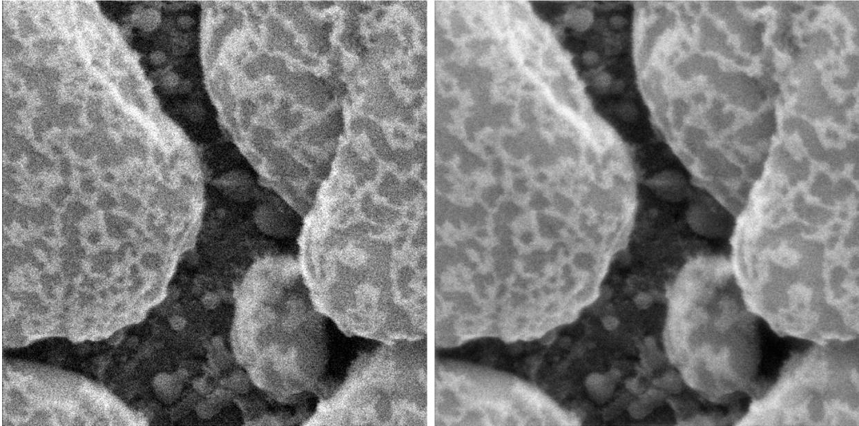
Figure 5. The result of a new NIST image processing method that can eliminate a part of the noise without significantly altering fine image details. Decorated gold on carbon sample, 1  $\mu\text{m}$  field-of-view.
