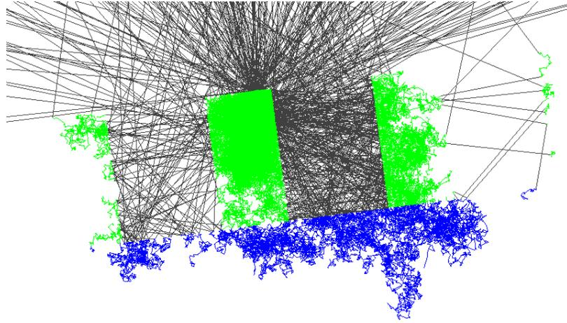
Figure 6. JMONSEL Simulation of 1 keV electron trajectories in a 7.5 degree tilted sample with 20 nm wide SiO<sub>2</sub> lines. Note that some of the electrons hit other neighboring lines' walls.
