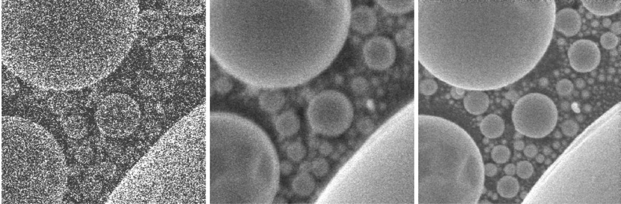
Figure 3. Single image acquired in 11  $\mu$ s frame time (50 ns pixel dwell time) (left). Traditionally averaged 70 images (middle). The same 70 images averaged with the new, adaptive method (right). The field-of-views are 4.6  $\mu$ m.
