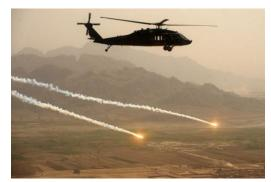
Figure 14. Large platform expending flares [25] Figure 15. Helicopter expending flares [26]
