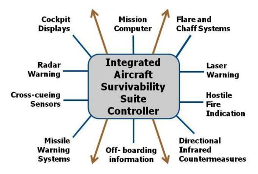
Figure 28. Integrated Aircraft Survivability Equipment Architecture
