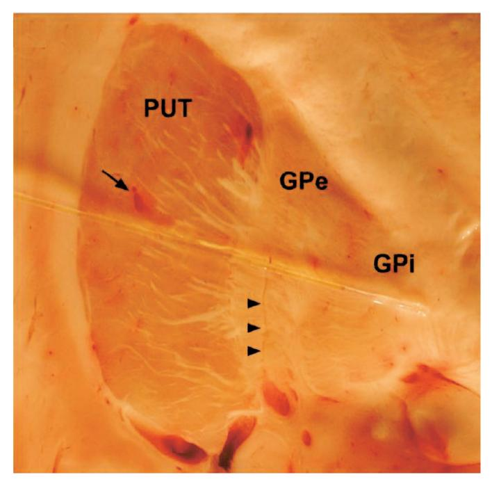
**Fig. 2** Actual catheter-based OCT imaging probe is placed on top of a brain section through the human putamen (PUT), globus pallidus externa (GPe), and globus pallidus interna (GPi). The tip of the probe is placed just past GPi. Its diameter is 0.36 mm. The arrows point to blood vessels that are discussed in the text.
