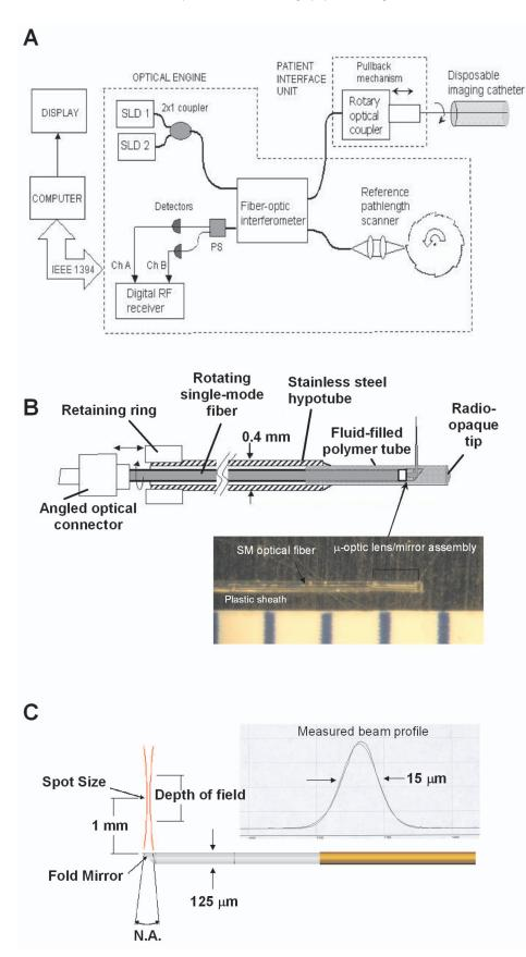
**Fig. 1** (a) Block diagram of the prototype OCT system, built by LightLab Imaging (Westford, Massachusetts) for neuroimaging research; (b) schematic of the imaging probe employed in this study, based on a fiber optic imaging core, and (c) schematic of the micro-optical lens/beam deflector assembly at the tip of the catheter, with a representative beam profile measured at the focal point of the microlens.
