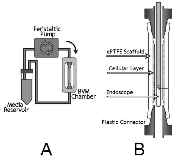
Fig. 2 Imaging of the BVM: (A) the bioreactor system and (B) schematic of BVM imaging geometry.
