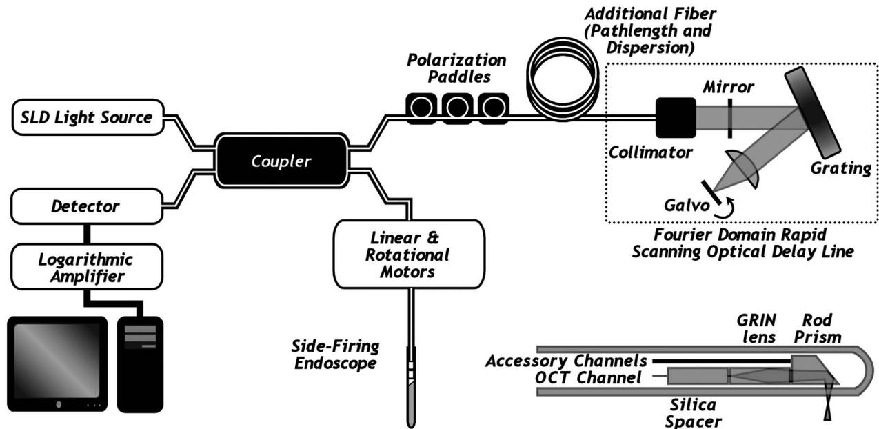
Fig. 1 Schematic diagram of the endoscopic OCT system.
