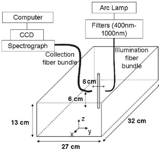
**Fig. 1** Experimental setup showing the container of the tissuelike liquid phantom and the cylindrical inclusion containing the two test chromophores. CCD: charge-coupled device.
