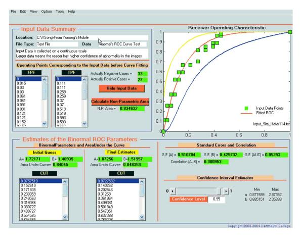
**Fig. 3** A screen view of the graphical user interface (GUI)-based ROC fitting platform is shown, which includes empirical nonparametric initial analysis, maximum-likelihood estimation-based binormal ROC analysis, and related statistical parameter analysis such as the ROC curve confidence interval boundary, standard error, data correlation, and parameter confidence intervals.
