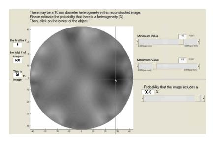
Fig. 2 The image detection program is shown. Observers can adjust the image gray map scale with the top two slide bars, and point to the estimated heterogeneity location with the computer mouse.
