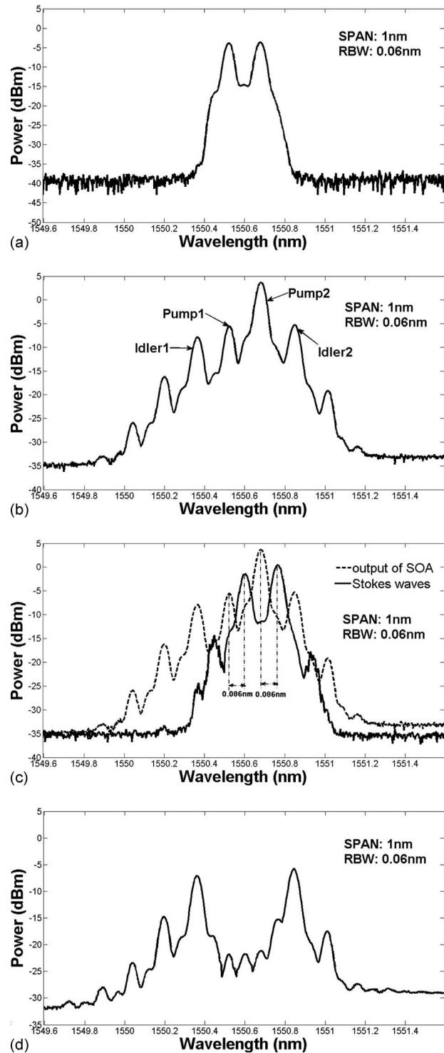
**Fig. 2** Measured optical spectra: (a) The signal after MZM, (b) after SOA with FWM, (c) contrast between the Stokes waves from BFL and the output from SOA, and (d) the generated mm-wave after pump suppression in the BFL.
