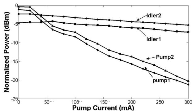
Fig. 3 Dependence of pumps; idlers on EDFA pump current.
