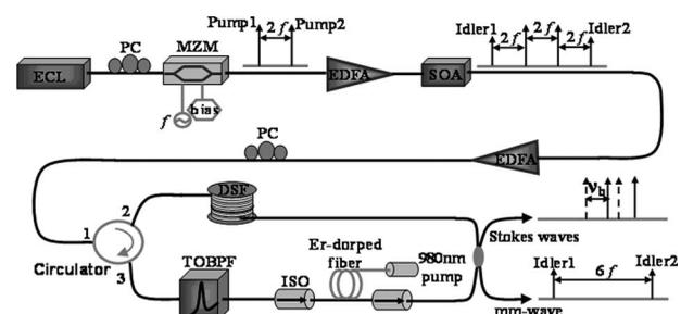
Fig. 1 Schematic diagram of mm-wave subcarrier generation.
