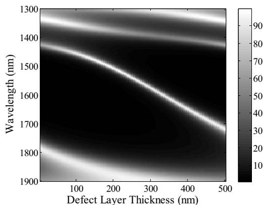
**Fig. 2** Continuous tuning of the transmission as obtained across the stop band was achieved. High transmission ( $>90\%$ ) and excellent sidelobe suppression was achieved throughout the tuning range. Color bar on the right indicates percent transmission.
