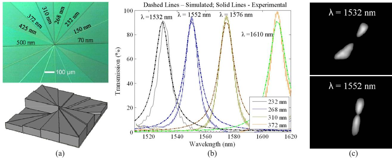
**Fig. 4** (a) Optical microscope image of the charge 2 vortex elements and schematic. (b) Simulated (dotted lines) and experimental transmission spectra. (c) Images of the spatial transmission through the vortex element at 1532 nm and 1553 nm. The vortex element was illuminated using a beam of diameter 3 mm.
