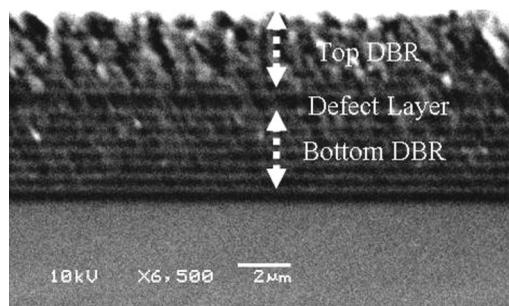
**Fig. 3** Cross-sectional scanning electron micrograph (SEM) of the fabricated multilayer stack obtained by cleaving through one of the diffractive levels. The layered structure consisting of nitride (lighter regions) and oxide (darker regions) layers with an oxide defect layer is clearly seen in the micrograph.
