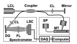
**Fig. 1** Schematic diagram of the SDODT. Incident light was inclined by 5 deg from the vertical. CL, collimating lens; DG, diffraction grating; FL; focusing lens; LCL, low coherent light; LSC, line scan camera; MT, microtube; SP, syringe pump; DAQ, data acquisition.
