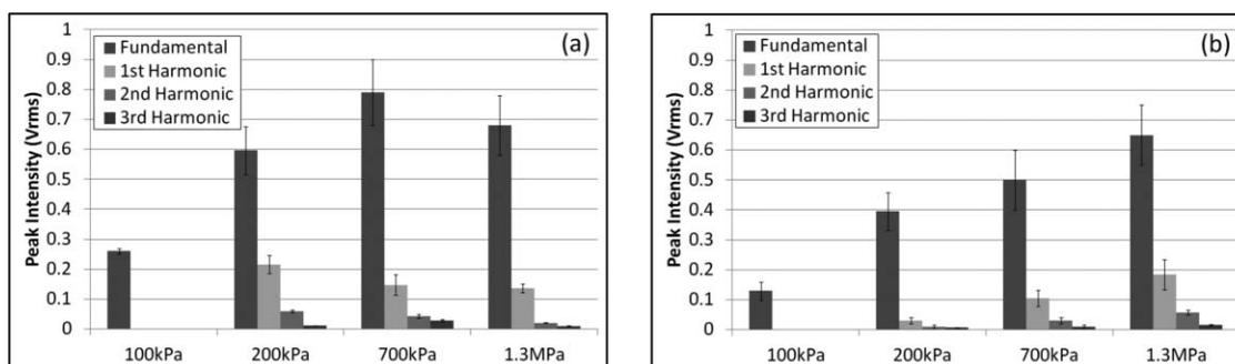
**Fig. 4** (a) Harmonic frequency peak intensity versus acoustic pressure for Definity and (b) albumin-shelled microbubbles.
