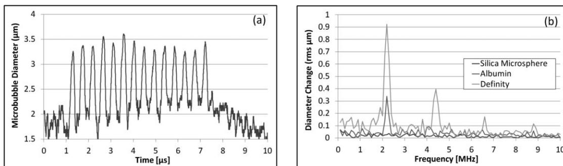
**Fig. 3** (a) Time domain waveform of asymmetric radial oscillation of Definity microbubble at 200 kPa. (b) Corresponding frequency response at 200 kPa of silica microsphere, albumin microbubble, and Definity microbubbles with the presence of higher harmonics.
