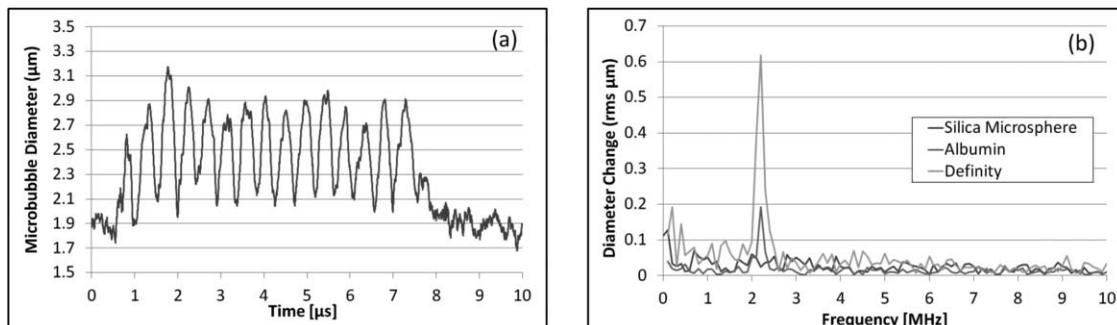
Fig. 2 (a) Time domain waveform of symmetric radial oscillation of Definity microbubble at 100 kPa. (b) Corresponding frequency response at 100 kPa of silica microsphere, albumin microbubble, and Definity microbubbles.
