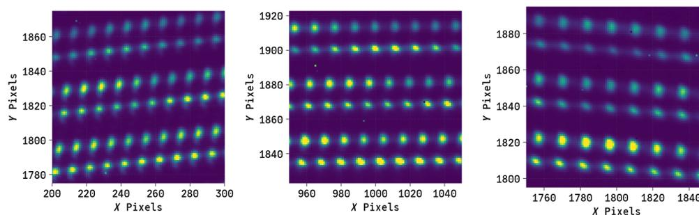
**Fig. 2** Raw PARVI frame of the LFC injected through the science (top) and calibration (bottom) fibers. We show the same three orders  $m = 89$  to 91 across the detector (top to bottom; wavelength increases from left to right). The tilt in the PSF is different for the two fibers and changes across each order (and orders). The colormap is arbitrarily scaled for adequate contrast.
