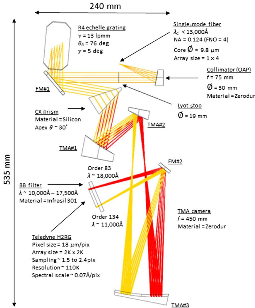
**Fig. 1** Schematic showing the layout of the cross-dispersed echelle spectrograph, which is designed to achieve  $R \sim 87,000$  to  $121,000$  in a compact  $0.5 \text{ m} \times 0.25 \text{ m}$  optical bench through the use of a SMF input from the Palomar AO system.
