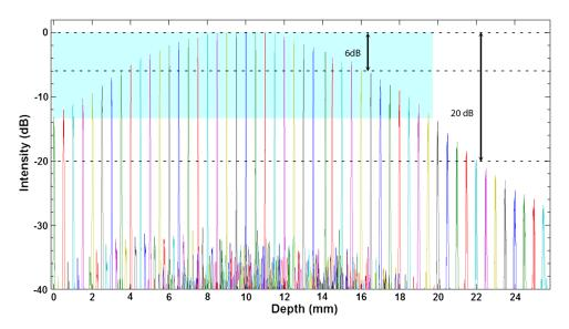
**Fig. 3** Sensitivity of the OCT system with respect to depth. The imaging ranges for 6 and 20 dB sensitivity roll off are 12.8 and 22.2 mm, respectively. For the symmetrical portion of the sensitivity roll off profile, the imaging range is 19.7 mm.
