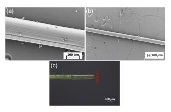
**Fig. 3** (a) and (b) SEM images of fiber. The fiber diameter is approximately 180  $\pm$  20  $\mu$ m. (c) Light microscope image of F-PVA fiber.
