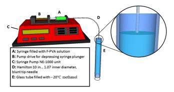
**Fig. 2** Setup for wet spinning of PVA/F-PVA fibers. A syringe containing the F-PVA solution is placed in a syringe pump and slowly injected into a glass tube filled with  $-20^{\circ}$ C methanol. The needle was positioned just above the methanol and was lowered until an interface formed. DMSO and water diffuse out of the fiber causing the now insoluble F-PVA to solidify.
