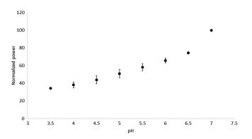
**Fig. 7** Transmittance of F-PVA fiber as a function of pH, in citrate buffer, pH 6.5, 6.0, 5.5, 5.0, 4.5, 4.0, and 3.5 using a 490-nm LED source and the perpendicular setup. As the pH decreased, transmittance decreased as well. Normalized values show the power at each pH as a percentage of the highest value achieved, which was at pH 7 for all fibers tested. n=3 and the error bars represent deviation from the mean.
