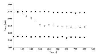
Fig. 6 Changes in transmittance with F-PVA fiber dry (•), wet (∘), and after HCI addition (pH 1) (■).
