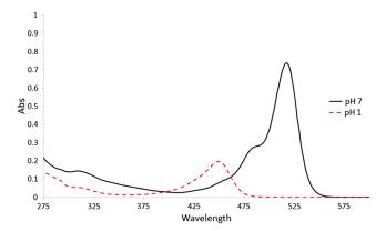
**Fig. 4** UV–Vis absorbance spectra of F-PVA in DMSO and HCl. Eleven milligram of spun F-PVA fiber was dissolved into 1 mL of DMSO. F-PVA at neutral pH (solid line) and F-PVA at in 0.1 M HCl (pH 1) (dashed line).
