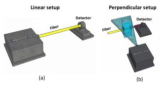
**Fig. 5** (a) Linear setup with the source opposite the detector. (b) Perpendicular setup with the source at a 90-deg angle to direction of the fiber. The linear setup is perfect for *in vivo* applications, whereas the perpendicular setup is viable for *in vitro* applications.
