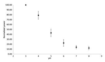
**Fig. 9** Normalized power of F-PVA fibers (n=4) using linear setup. The highest variability was seen at pHs 4 to 6, where the sensitivity of fluorescein is greatest. Normalized values show the power at each pH as a percentage of the highest value achieved, which was at pH 3 for all fibers tested. Error bars represent the deviation from the mean.
