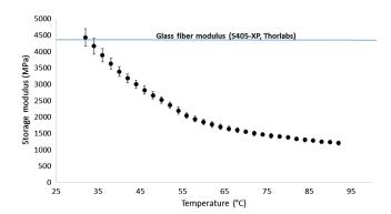
**Fig. 10** DMA testing results of a dry F-PVA fiber (n=4). Peak storage modulus was about 4000 to 5000 MPa, which declined with increasing temperature to about 1200 MPa at 95°C. A glass transition temperature can be seen at about 55°C. n=3, and the error bars represent the deviation from the mean.
