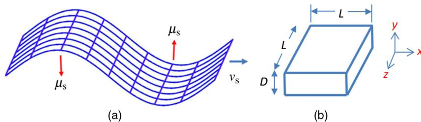
**Fig. 1** (a) A TIESW on the surface of a squared slab of isotropic and homogeneous viscoelastic medium in (b).
