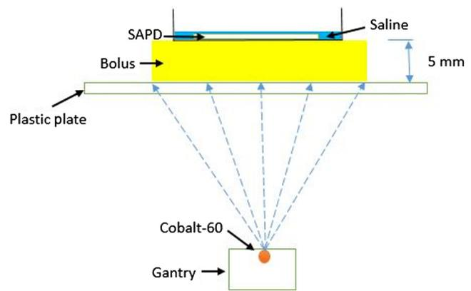
**Fig. 7** Geometry of inverted incidence of the ionized radiation beam.
