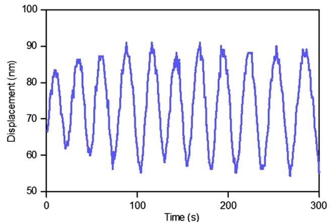
**Fig. 11** TIESW profile of a SAPD 24 h after being exposed to radiation under highly absorbed dose with permanent damage.
