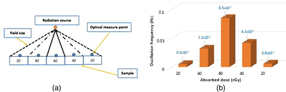
**Fig. 12** (a) Setup of 1-D dose distribution in an SAPD at a given exposure of ionizing radiation and (b) the measured 1-D absorbed dose distribution versus TIESW oscillation frequency.
