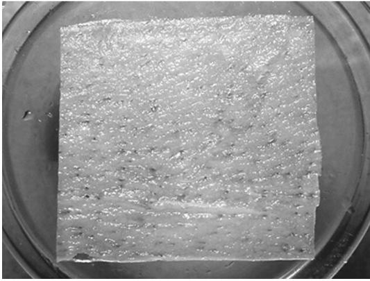
**Fig. 3** Picture of squared SAPD with a 25-mm width and 0.5-mm thickness.
