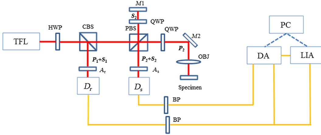
**Fig. 2** Optical setup of TFPPI. TFL, two-frequency laser; HWP, half wave plate; QWP, quarter wave plate;  $A_r$ ,  $A_s$ , analyzers;  $D_r$ ,  $D_s$ , detectors; BP, band pass filter; OBJ, objective lens; DA, differential amplifier; LIA, lock-in amplifier.
