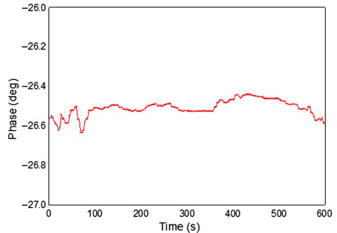
**Fig. 4** Differential-phase stability of TFPPI.
