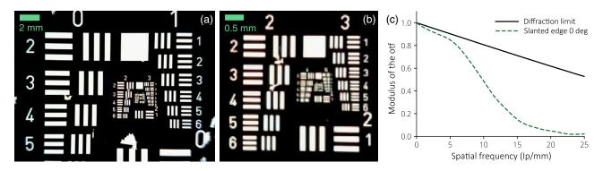
**Fig. 3** Image of a 1951 USAF resolution test chart showing (a) the 15 mm × 20 mm FOV and (b) contrast limit. The zoomed contrast limit image (b) shows group 4–3 is resolvable, a cutoff frequency of 20.16 lp/mm. (c) A comparison of the theoretical diffraction limit and measured on-axis MTF performance.
