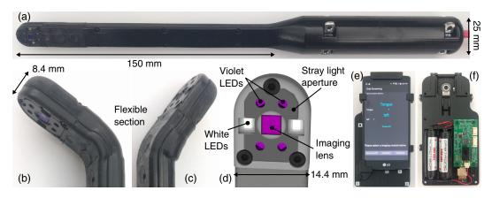
**Fig. 1** Intraoral probe system view showing the handheld probe: (a) overall system size; (b), (c) the flexible head; (d) the imaging and LED illumination apertures, along with the (e) installed smartphone running the custom Android application and (f) installed electronics.
