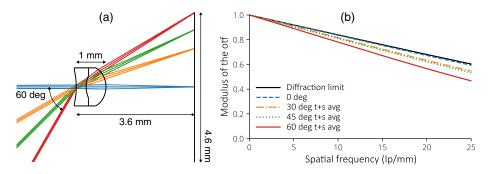
**Fig. 7** Optical design for a 120-deg full FOV, image space NA = 0.023 lens with increased MTF performance compared to Fig 3. (a) The layout of the optical design with dimensions; (b) provides the theoretical MTF performance.
