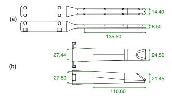
**Fig. 6** Comparison of mechanical outlines for (a) the probe proposed in this paper and (b) the previously published probe<sup>9</sup> demonstrating its greatly reduced intraoral dimensions.
