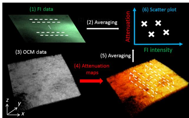
**Fig. 2** The data processing pipeline. First, OCM and FI images are acquired. Attenuation maps are generated from the OCM data. Attenuation coefficients are averaged in a chosen region of interest. The results from the attenuation analysis are then compared in a scatter plot with their respective averaged FI values.
