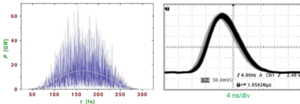
Fig. 3 FEL pulse by simulation and measured LPP pulse of 4-ns FWHM.
