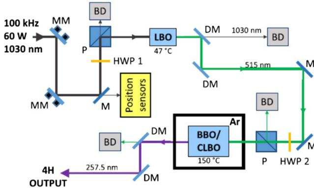
**Fig. 8** Optical arrangement in the second and fourth harmonics generation. MM, motorized mirror; M, mirror; BD, beam dump; HWP, half wave plate; DM, dichroic mirror; P, polarizer.
