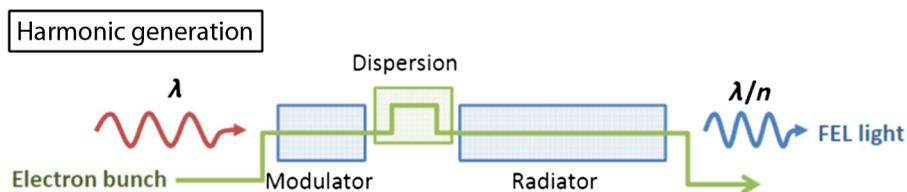
Fig. 4 External seeding for controlled FEL pulses.
