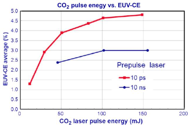
**Fig. 1** CE dependent on input CO<sub>2</sub> pulse energy with prepulse of ns and ps.
