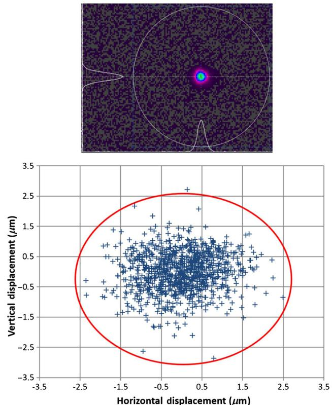
**Fig. 6** Beam shape and pointing stability from 1-kHz thin-disc regenerative amplifier.
