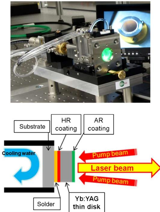
**Fig. 5** Thin-disc module and cross section of the thin-disc core region.
