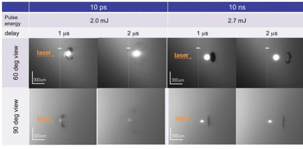
Fig. 2 Dispersion dynamics of tin droplet by ps and ns pulses.
