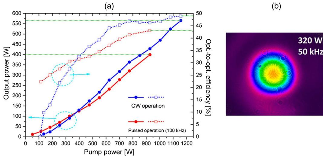
**Fig. 7** (a) Average output power and O–O (optical–optical) efficiency of the main regenerative amplifier versus pump power and (b) beam profile at 320 W, 50 kHz.
