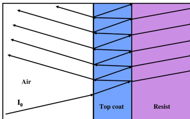
Fig. 15 Light path of top coat/antireflective coating and resist film stack.<sup>43</sup>
