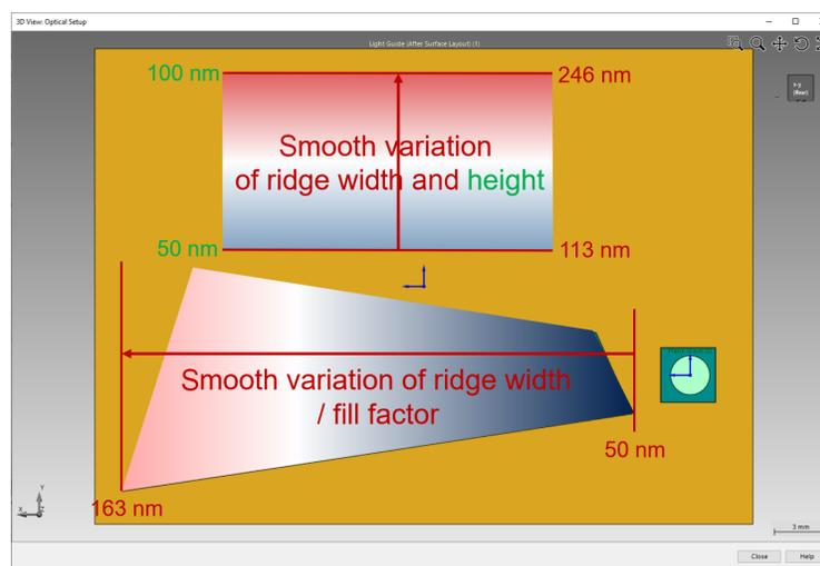
**Fig. 2** Depiction of the modulation of grating parameters in the EPE and outcoupler with results obtained through parametric optimization.
