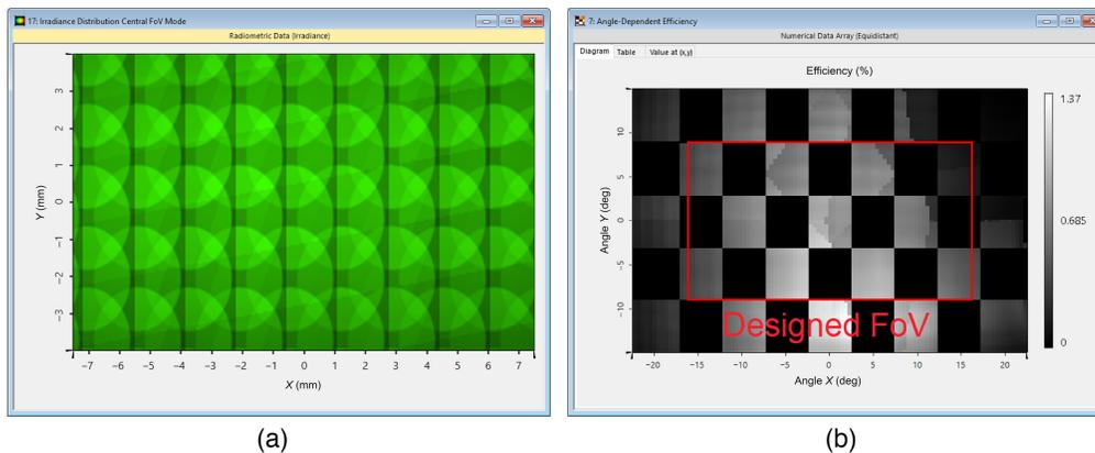
**Fig. 3** (a) Irradiance distribution in the eyebox for the central mode of the FoV (0.86% efficiency, 20.2% lateral uniformity error) obtained by physical optics modeling in a real color view. (b) Angle-dependent distribution of the efficiency of the designed waveguide in the whole FoV (area of interest) and beyond, evaluated by a checkerboard pattern in angular coordinates (0.62% mean efficiency, 82.0% angular uniformity error).
