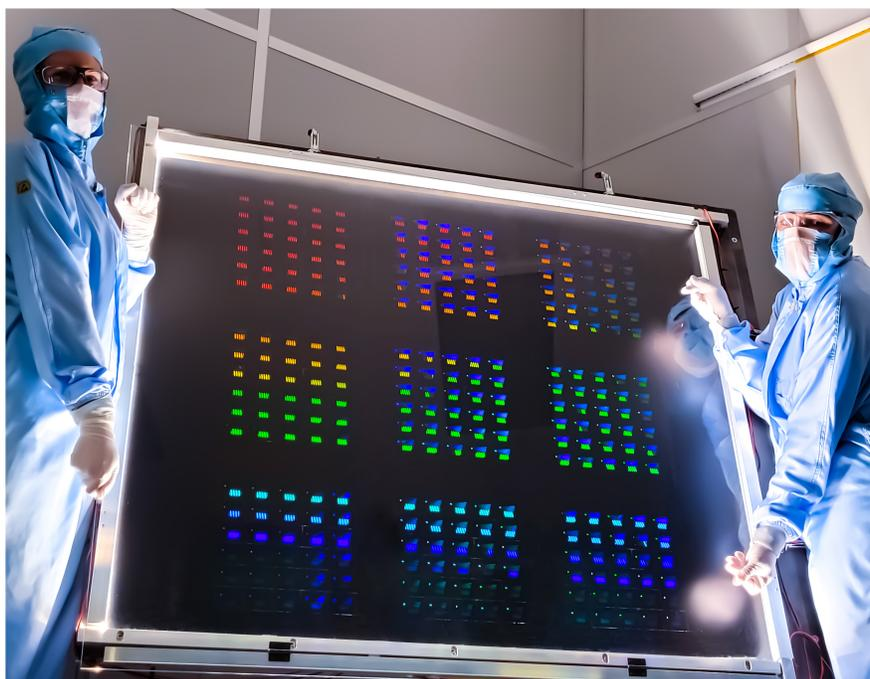
**Fig. 6** Replication of the 30-up scaled-up sub-master on 9 single wafers producing 270 waveguides in one imprint pass.
