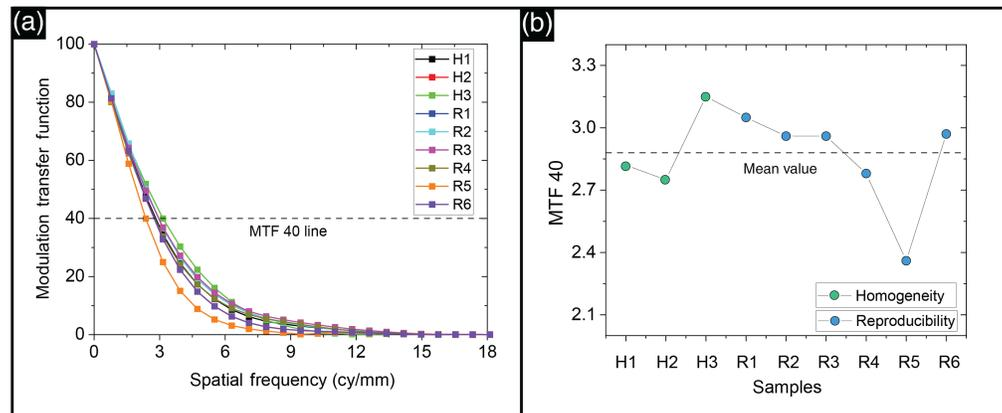
**Fig. 11** (a) MTF graphs for all samples versus spatial frequency, H1 to H3 are selected tiles from single imprint number 1, and R1 to R6 are imprints 2, 11, 50, 70, and 101. (b) MTF of 40% is shown for all imprints and tiles for a closer comparison.
