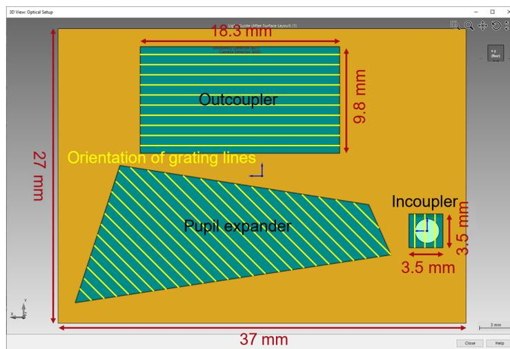
**Fig. 1** Top view of the lateral layout of the designed waveguide. The orientations of the grating lines are indicated in green.
