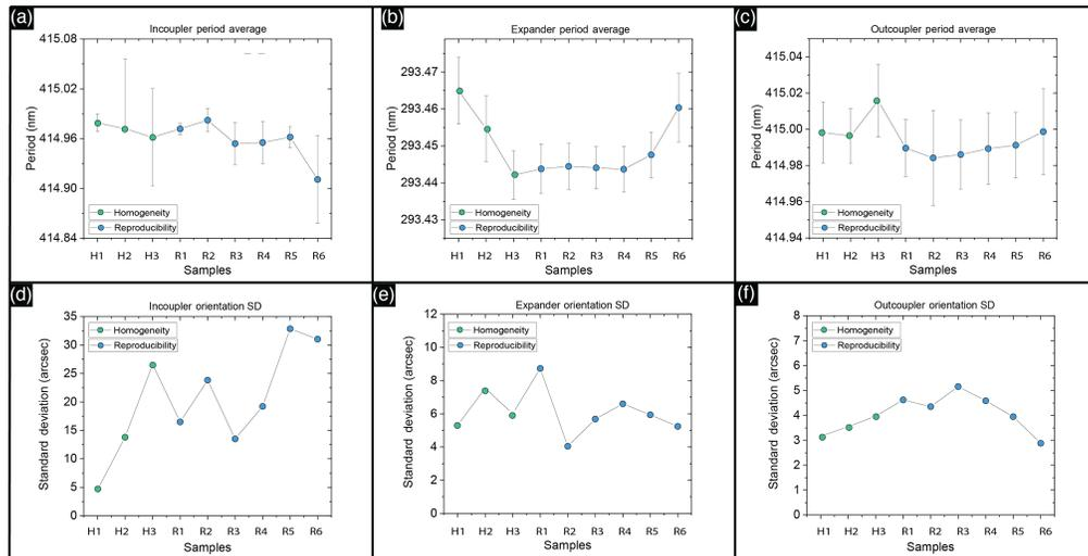
**Fig. 9** (a)–(c) Average period with standard deviation of each grating. The graph shows that the average period is similar from sample to sample. (d)–(f) Standard deviation of the relative orientation of the grating lines. Incoupler SD presents a low reliability due to small number of measurement points.
