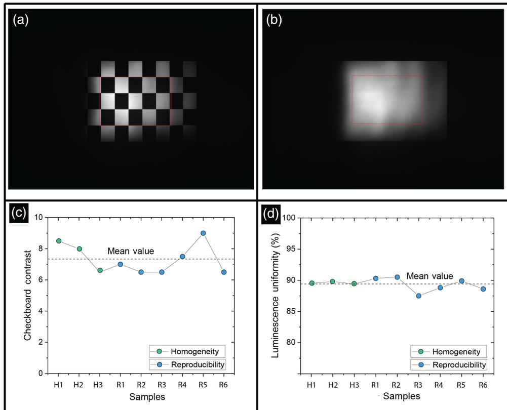
**Fig. 10** Regions of interest for analyzing the waveguide images based on the FoV of the test waveguides are shown as a red frame for both (a) checkerboard and (b) solid reticles. For both groups of the homogeneity (H1 to H3) and reproducibility (R1 to R6) waveguides, the analysis results of the checkerboard contrast and luminescence uniformity are presented in panels (c) and (d), respectively.
