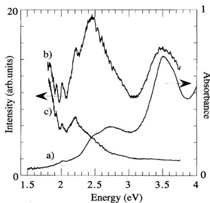
**Fig. 4** (a) UV/visible absorption, (b) luminescence excitation (monitoring at 1.66 eV) and (c) luminescence efficiency spectra ( $T = 77$  K, annealed C<sub>60</sub> film, 20 nm). Reproduced with permission from Ref. 38. Copyright © 1995 by the American Physical Society.
