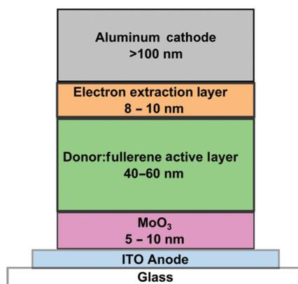
**Fig. 2** General structure of a Schottky junction OSC with typical thicknesses of layers reported in literature.
