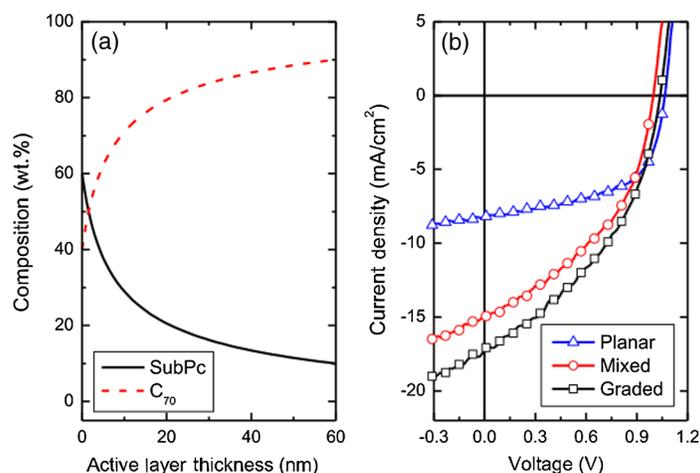
**Fig. 3** (a) Graded doping profile of SubPc: $C_{70}$  devices with an overall  $C_{70}$  concentration of 80% and (b) I-V curves under  $134 \text{ mA/cm}^2$  AM1.5G irradiation for a planar junction device (11 nm SubPc/35 nm  $C_{70}$ ), a uniformly mixed 20% SubPc:80%  $C_{70}$  device and a graded 80%  $C_{70}$  device. Reproduced with permission from Ref. 31. Copyright © 2012 by American Institute of Physics.
