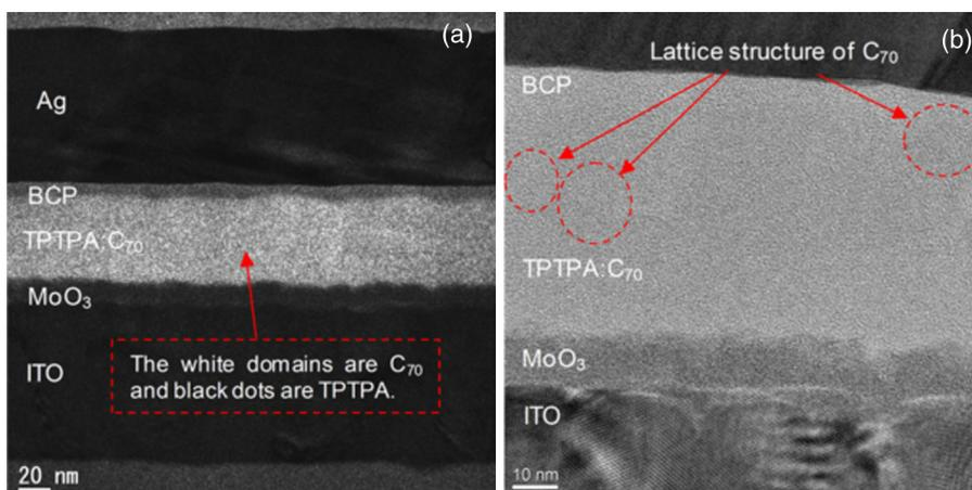
**Fig. 9** (a) Energy-field mode and (b) bright-field mode cross-sectional TEM images of 5% TPTPA:C<sub>70</sub> OSCs showing extensive phase separation between C<sub>70</sub> and TPTPA. Reproduced with permission from Ref. 28. Copyright © 2013 by American Institute of Physics.
