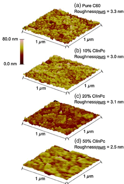
**Fig. 7** AFM images of (a) neat  $C_{60}$  film, (b) 10% CInPc in  $C_{60}$ , (c) 20% CInPc in  $C_{60}$ , and (d) 50% CInPc in  $C_{60}$ . Reproduced with permission from Ref. 25. Copyright © 2013 by Elsevier B.V.
