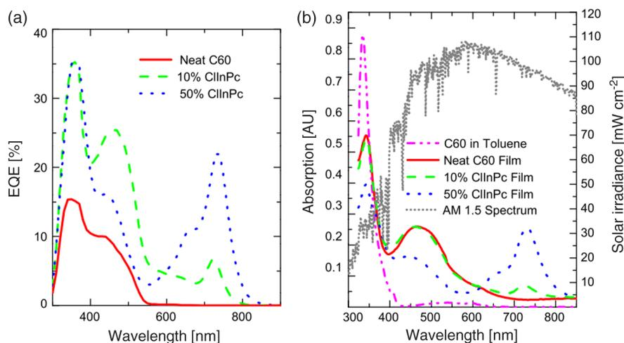
**Fig. 6** (a) EQE spectra of CIInPc:C<sub>60</sub> Schottky OSCs with varying CIInPc concentration and (b) UV/Vis absorption spectra of the same. Also shown: UV/Vis absorption spectrum of C<sub>60</sub> and the AM1.5G spectrum. Reproduced with permission from Ref. 25. Copyright © 2013 by Elsevier B.V.
