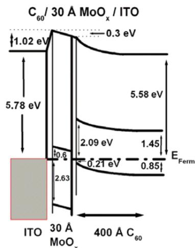
**Fig. 1** Energy level diagram of the  $\text{ITO}/\text{MoO}_3/\text{C}_{60}$  interface as determined using UPS and IPES. Reproduced with permission from Ref. 21. Copyright © 2011 by Elsevier B.V.
