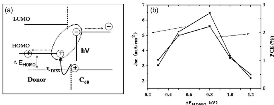
**Fig. 8** (a) Schematic of exciton dissociation in a Schottky OSC doped with donor material and (b) optimal  $\Delta E_{\text{HOMO}}$  for  $\text{C}_{60}$  intermolecular CT exciton dissociation. Reproduced with permission from Ref. 29. Copyright © 2013 by Elsevier B.V.
