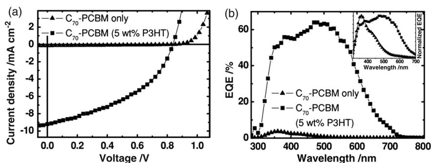
**Fig. 5** (a) I-V curves and (b) EQE spectra of neat  $PC_{70}BM$  and 5% P3HT: $PC_{70}BM$  OSCs. Reproduced with permission from Ref. 36. Copyright © 2012 by WILEY-VCH Verlag GmbH & Co.
