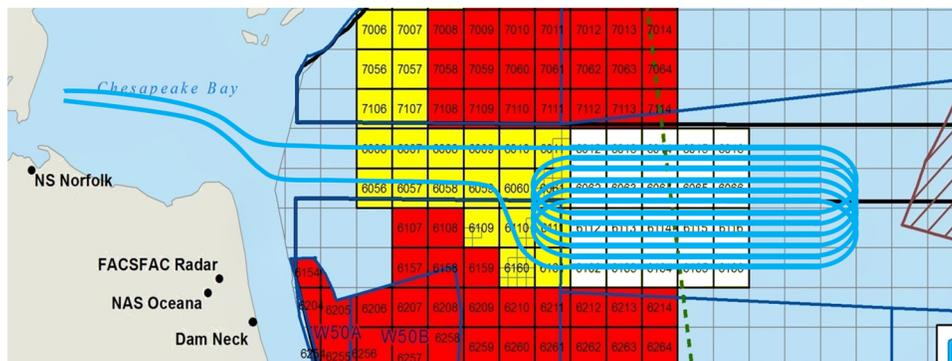
**Fig. 3** Map of the Virginia offshore wind energy area (WEA). The WEA is composed of 20 outer continental shelf blocks, shaded white in this map. Red shaded areas are warning areas of restricted air space. The notional aircraft flight path is drawn as a blue line.
