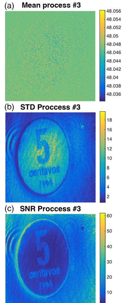
**Fig. 4** The maps represent (a) the mean value and (b) STD for each pixel of the frames calculated along the whole sequence (398 frames) obtained for the third class (P3) of the coin data set. (c) SNR is calculated as the ratio between the mean and STD for each pixel. Hidden topography is revealed from the STD and signal-to-noise maps.
