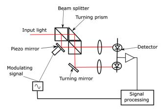
Fig. 1 Schematic diagram of the interferometer.
