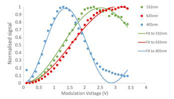
Fig. 6 Signal strength variation with modulation amplitude for laser light at 635, 532, and 405 nm.
