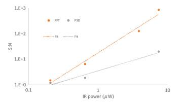
Fig. 3 Sensitivity measurements for the near IR version using 1.5  $\mu$ m light.
