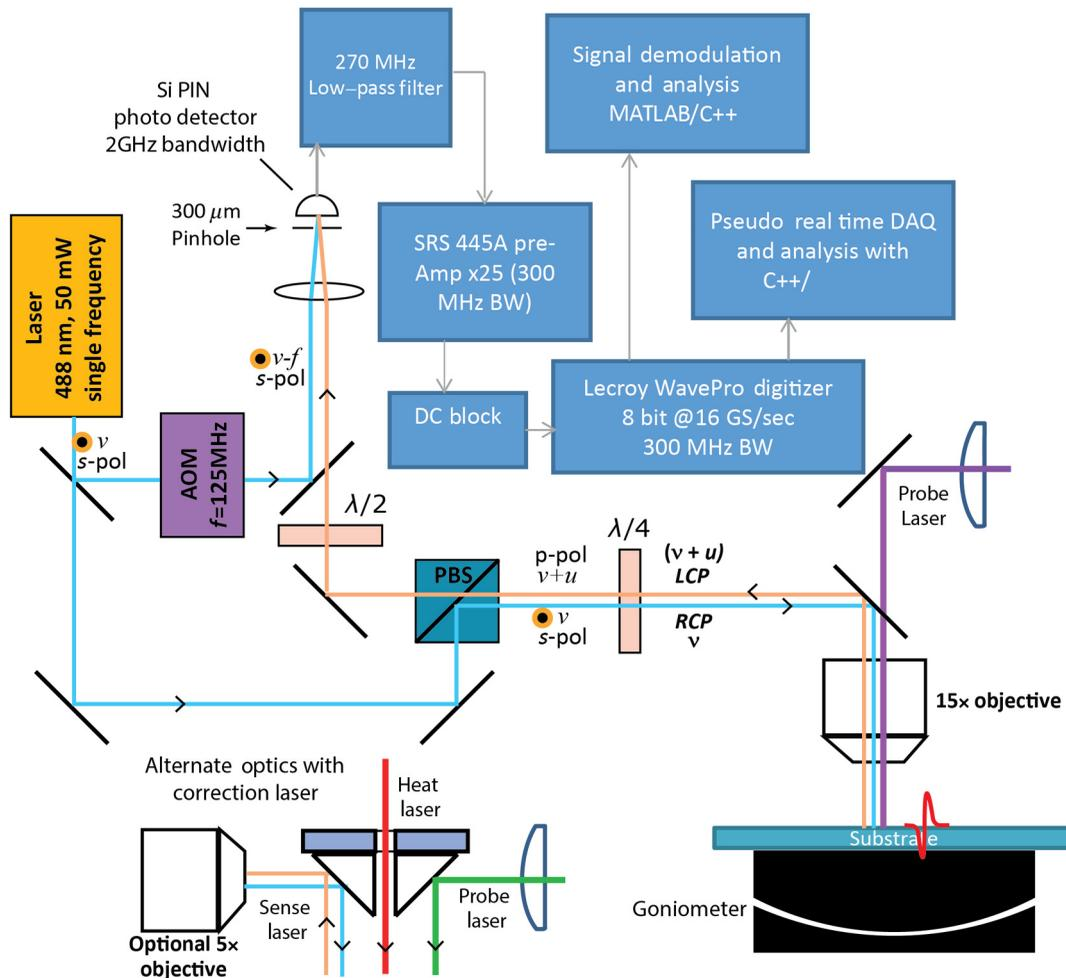
**Fig. 1** Experimental setup. Shows schematic of optical heterodyne system, guiding assembly for laser beams onto substrate, and block diagram of data acquisition chain.
