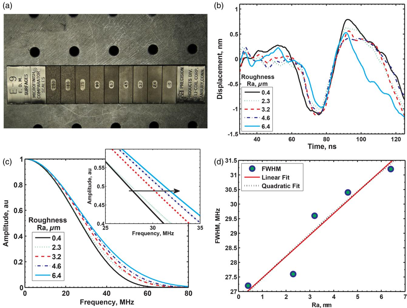
**Fig. 4** (a) GAR Electroforming E-9 electrical discharge machined microfinish comparator used for surface roughness evaluation. (b) Displacement versus time for SAWs measured over different roughness regions. (c) Frequency distribution (normalized with respect to the maximum) for the SAW waves measured over different surface roughness regions. (d) Frequency at the FWHM for the frequency distributions over each surface roughness region.
