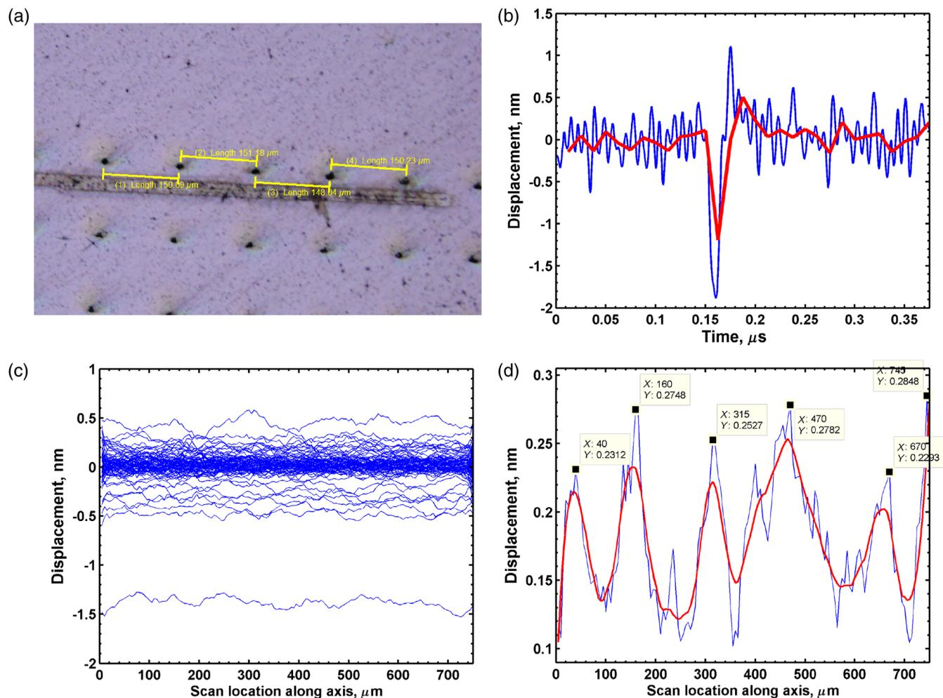
**Fig. 5** (a) Pre-fabricated square array of 10- to 20- $\mu\text{m}$  size holes separated by 150 microns in each direction. (b) SAW curve of a single probe–sense signal located at some location along the scan direction. (c) The displacement (itself a function of the time) versus the location along the scan axis. Each blue curve represents a different time point during recording of the surface measurements. (d) Filtering and peak extraction of a single displacement versus scan location curve.
