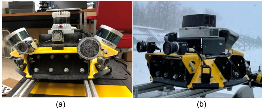
**Fig. 2** (a) Our IPEA system (sensor pod)<sup>8</sup> after year 2 testing campaign<sup>9</sup> mounted on a Husky A-200 robot with a 64-channel OS1 LiDAR unit at the top, a color camera on the left, an NIR camera on the right, and an LWIR camera in the middle. (b) The sensor pod was mounted on a test vehicle with a 905-nm MEMS LiDAR unit in our year 3 testing campaign.
