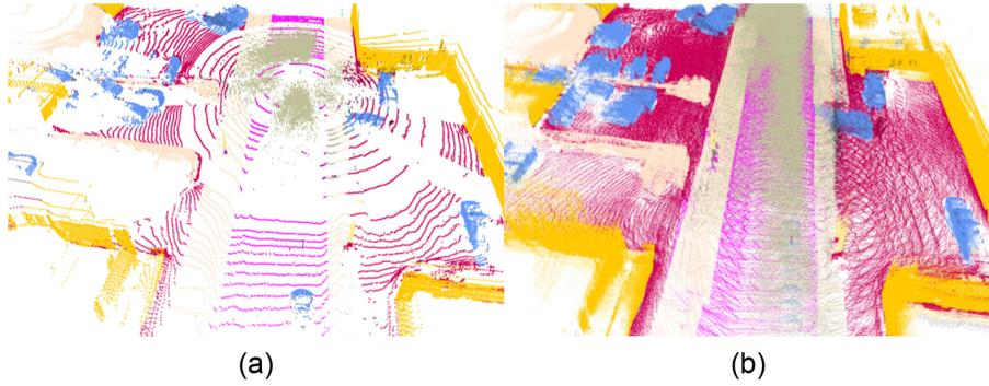
**Fig. 8** (a) A single labeled scan showing active falling snow and accumulated snow. (b) Several scans have been labeled and superimposed using pose information enabling spatial scene understanding.
