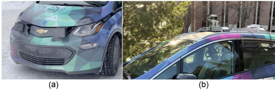
**Fig. 3** Our AV surrogate platform with the forward facing RADAR (a) mounted on the front bumper and a LiDAR (b) mounted on top of the vehicle.
