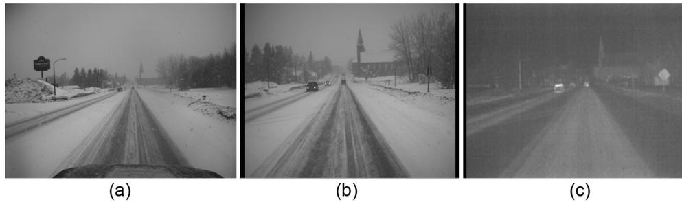
**Fig. 7** Example images collected during snowfall rates around 1 in (2.5 cm) per hour. The visible imagery (a) and NIR (b) show visible snowflakes, whereas the LWIR imagery (c) shows no effect of snowflakes.
