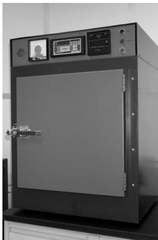
Figure 3. A vapor prime oven from Yield Engineering Systems. 3
