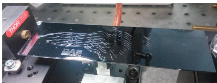
**Fig. 4.** Picture of the optical Butler matrix chip in the characterization set-up before packaging
