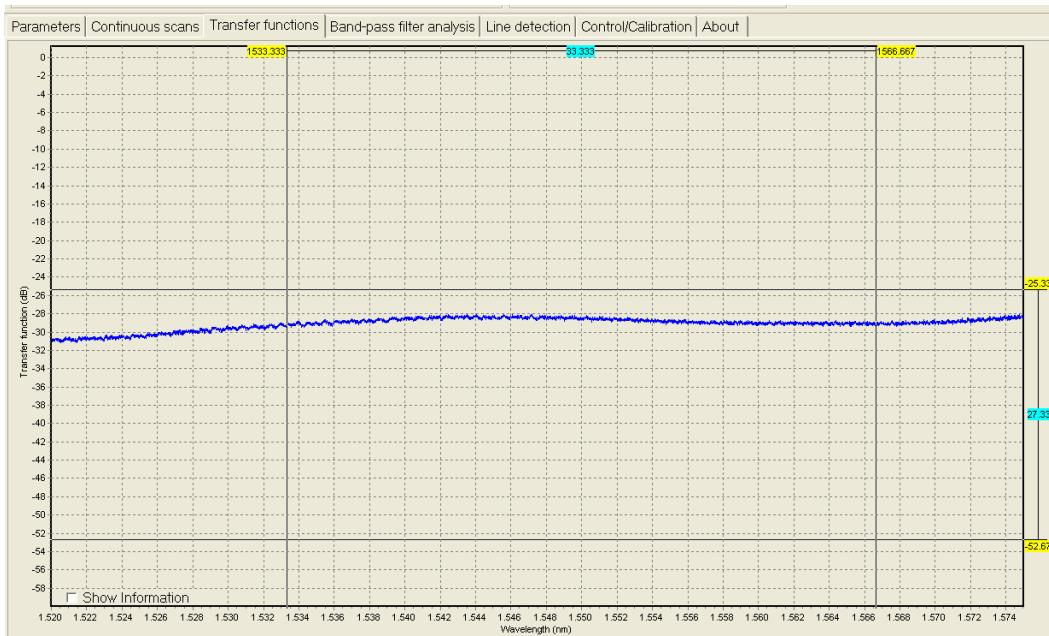
**Fig. 7.** Optical Power vs wavelength for TM polarization
