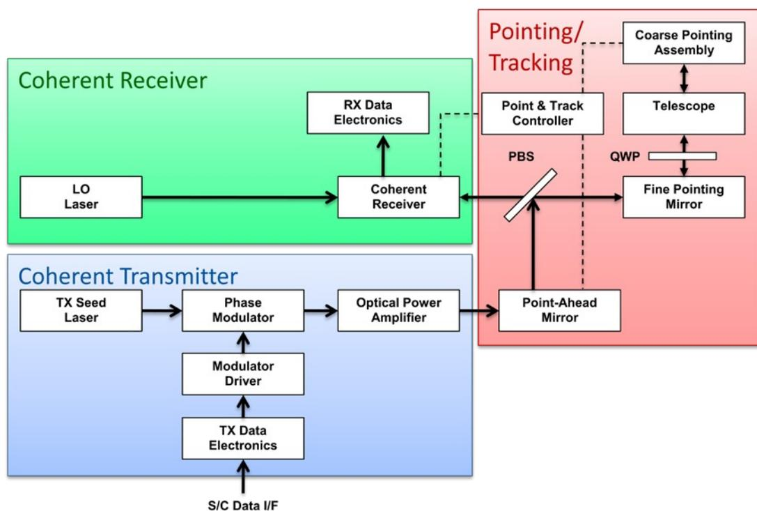
Fig. 1. LCT block diagram.
