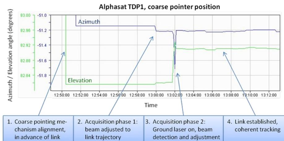
Fig 3: beam steering mechanism position during link acquisition
