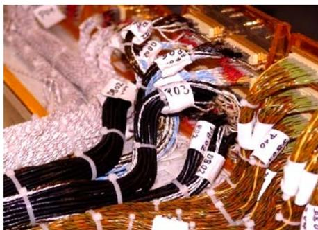
**Fig. 1:** Cable harness of a satellite with point-to-point wiring results in a complex cable harness.
