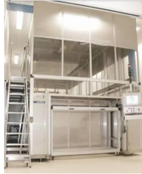
Fig.3. Automatic cleaning machine for large components
