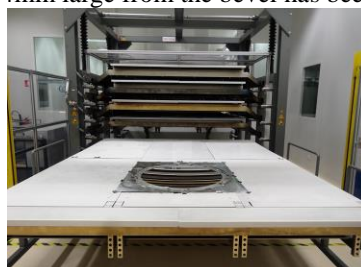
Fig.14. Coated M1 Mirror on the tray (Zerodur®, 591mm diameter)
