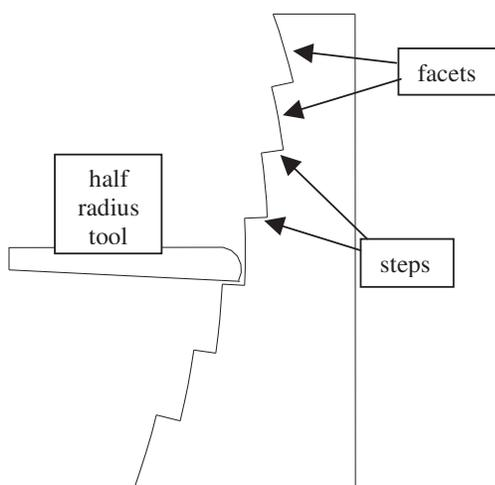
Fig. 6 Slicer schematic: cutting problem
