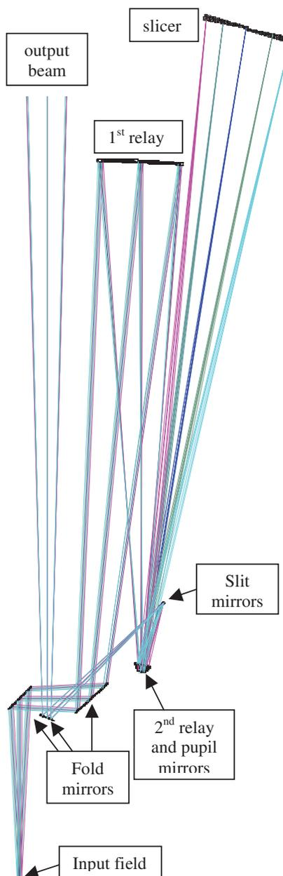
Fig. 2 Baseline optical design – view on YZ plane
