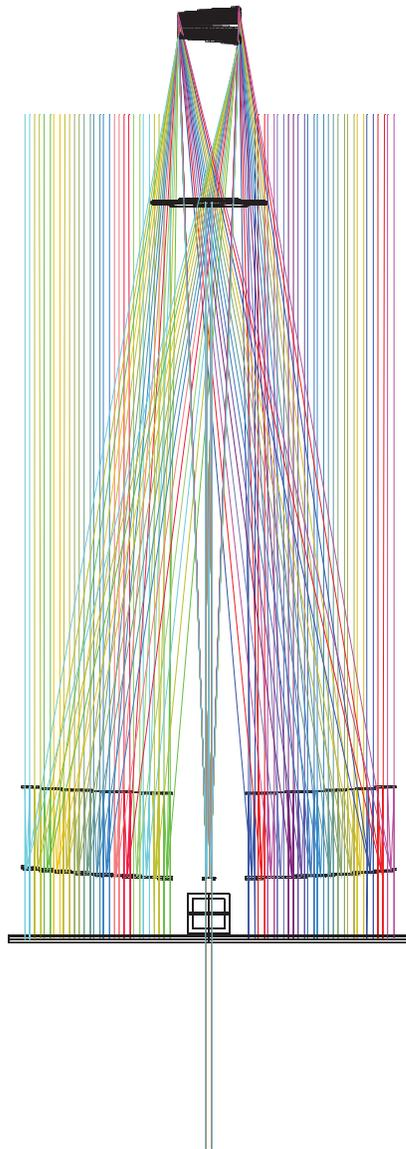
Fig.3 Baseline optical design – view on XZ plane
