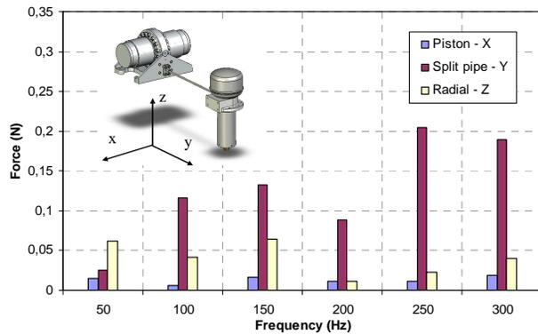
Fig. 3. EQM MPTC self induced forces at compressor interface - 50Wac input - 80K
