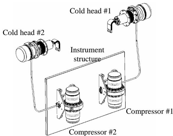
Fig. 4. MPTC redundant architecture integration
