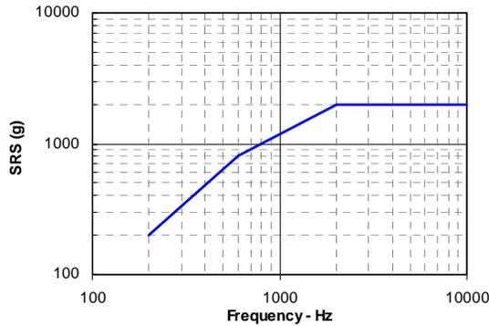
Fig. 8. shock load qualification profile
