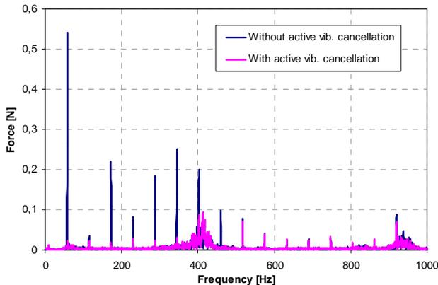
Fig. 12. EQM LPTC S/N002 self induced forces at compressor interface – 160 Wac input – 50K
