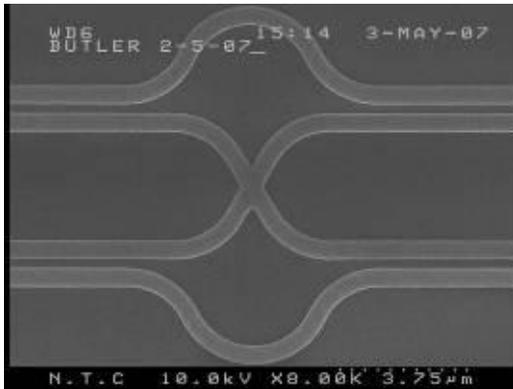
Fig. 2.- SEM Image of the 4x4 Photonic Butler Matrix
