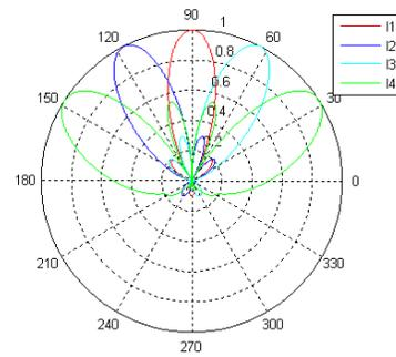
Fig. 3.-Theoretical radiation diagrams of an array of 4 antennas placed behind the beamforming unit.
