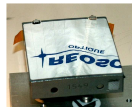
Fig (7): Coated COM with grounding straps
