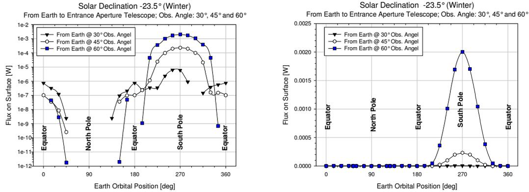
Fig. 4. Straylight originating from Earth illuminating the telescope entrance aperture (log. and lin. scale).
