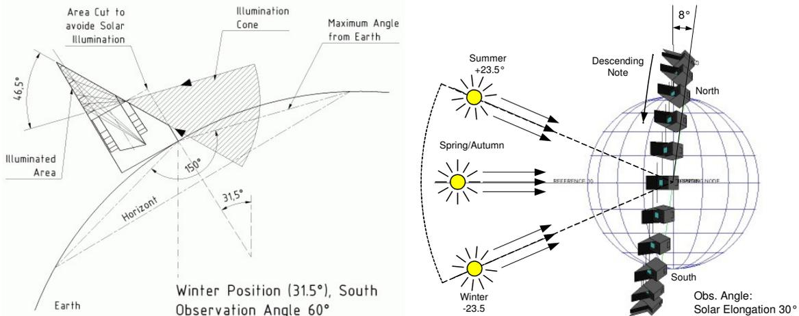
Fig. 3. AsteroidFinder geometrical model; orbit view with solar illumination.
