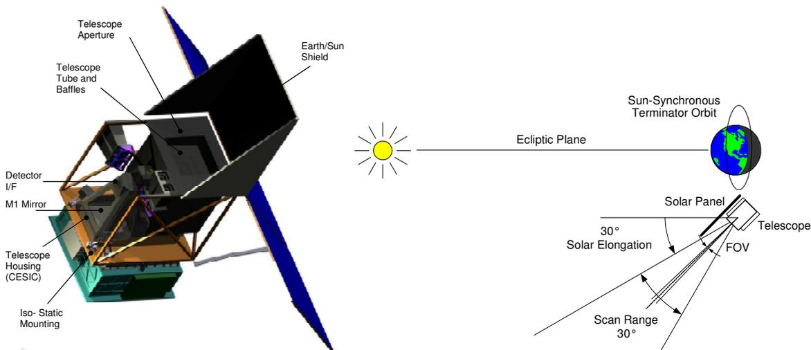
Fig. 1. AsteroidFinder model, orbit and proposed scan configuration.
