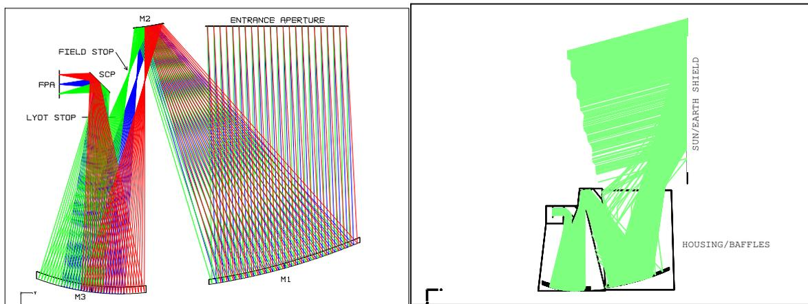
Fig. 5. Layout of the optical design; baffle geometry for the straylight analysis.
