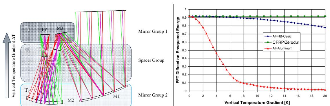
Fig. 6. ZEMAX<sup>®</sup> model comprising a simplified thermal model; optical performance analysis.
