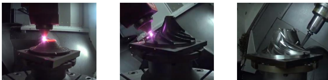
Figure 6 – 5-Axis Simultaneous 3D Additive Hybrid Manufacturing (Photos Courtesy of Jeffery Crandall - CCAT)
