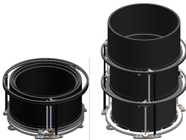
Figure 4: The deployable telescopic barrel, stowed (left) and deployed (right)
